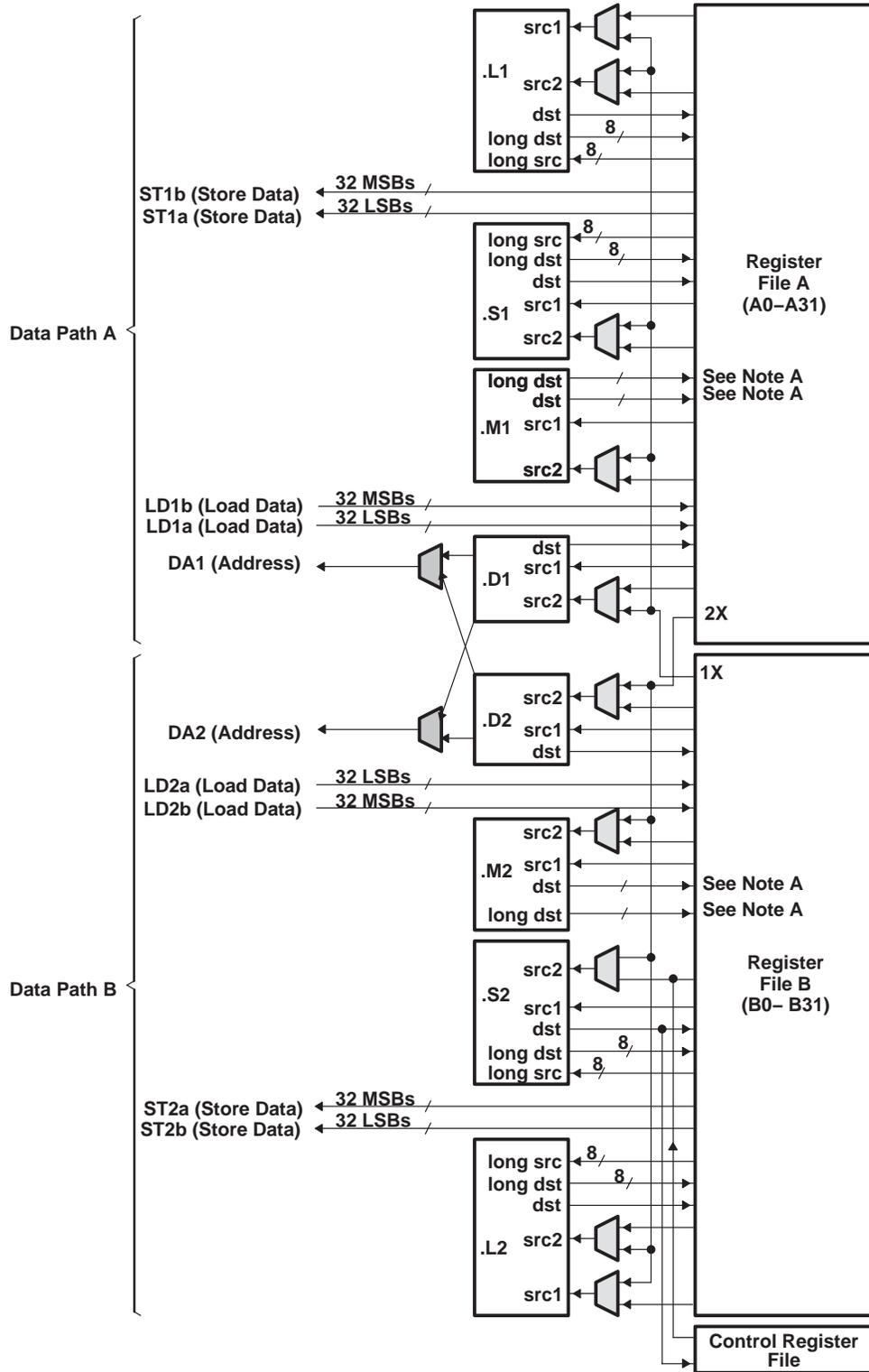
NOTE A: For the .M functional units, the long dst is 32 MSBs and the dst is 32 LSBs.
