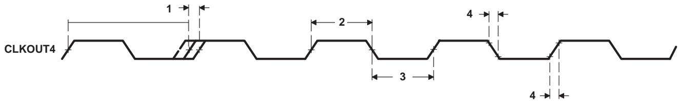
Figure 17. CLKOUT4 Timing
