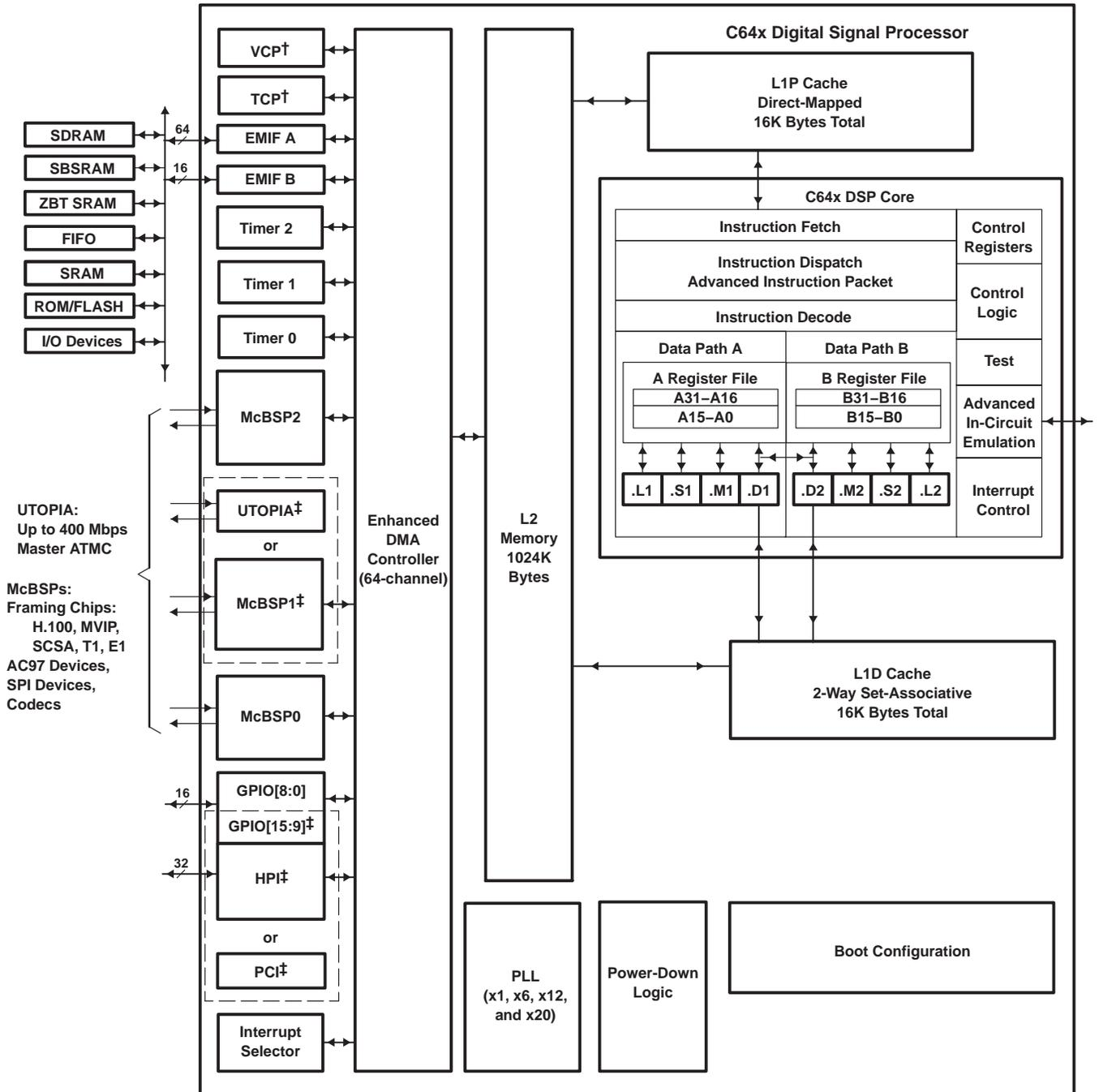
† The UTOPIA peripheral is MUXed with McBSP1, and the PCI peripheral is MUXed with the HPI peripheral and the GPIO[15:9] port. For more details on the multiplexed pins of these peripherals, see the Device Configurations section of this data sheet.
