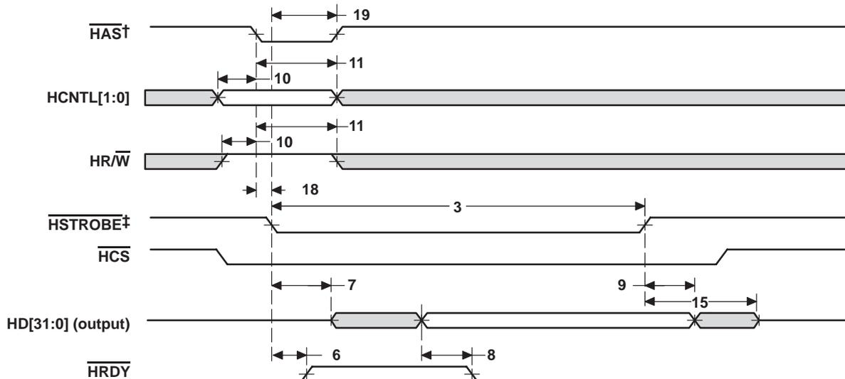
$^\dagger$  For correct operation, strobe the  $\overline{\text{HAS}}$  signal only once per  $\overline{\text{HSTROBE}}$  active cycle.
