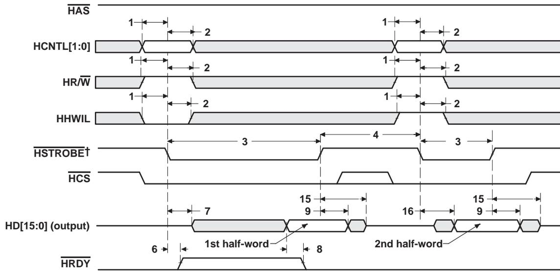
†  $\text{HSTROBE}$  refers to the following logical operation on  $\overline{\text{HCS}}$ ,  $\overline{\text{HDS1}}$ , and  $\overline{\text{HDS2}}$ :  $[\text{NOT}(\overline{\text{HDS1}} \text{ XOR } \overline{\text{HDS2}})] \text{ OR } \overline{\text{HCS}}$ .
