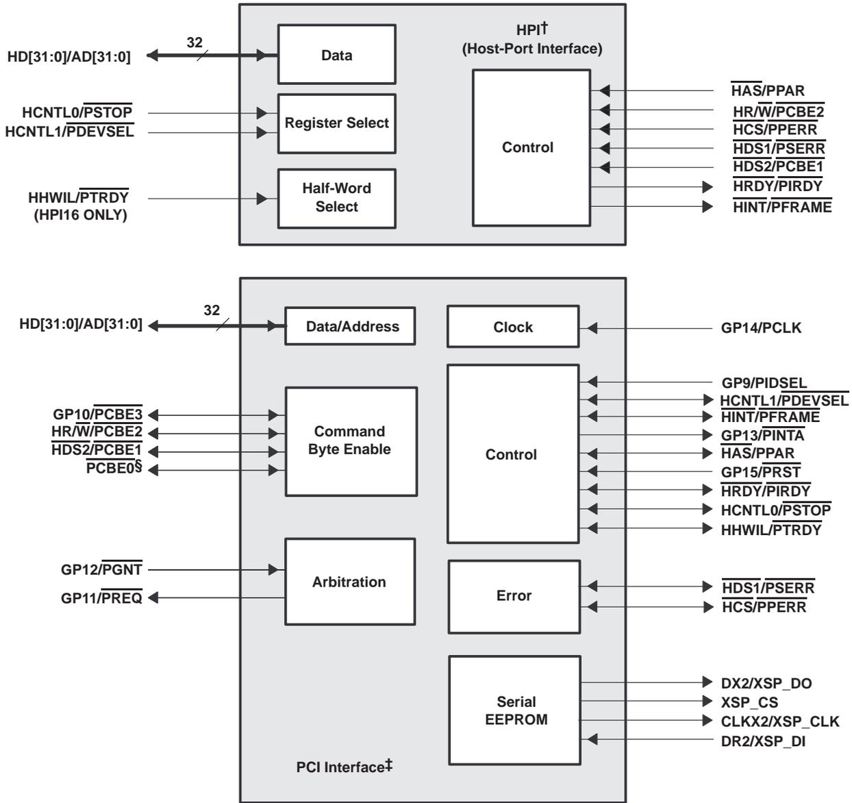
† These HPI pins are MUXed with the PCI peripheral. By default, these signals function as HPI. For more details on these MUXed pins, see the Device Configurations section of this data sheet.
