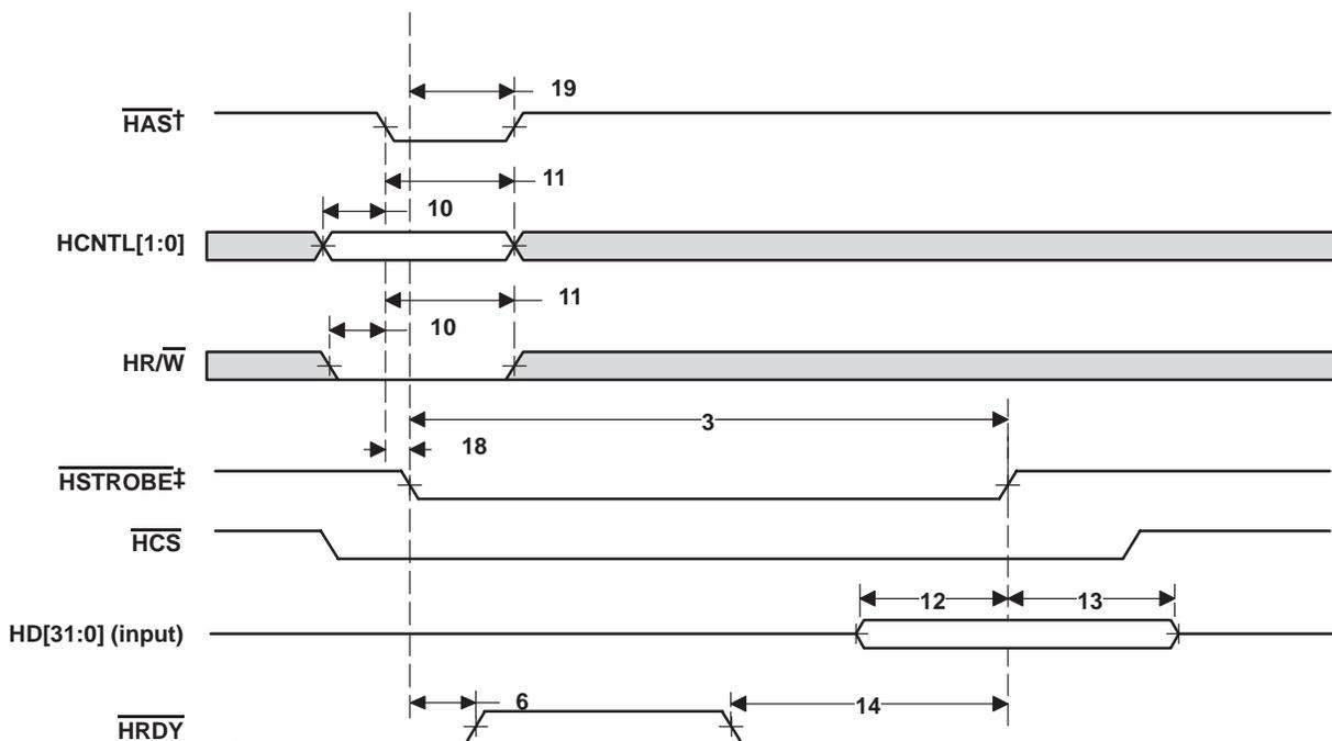
† For correct operation, strobe the  $\overline{\text{HAS}}$  signal only once per  $\overline{\text{HSTROBE}}$  active cycle.
