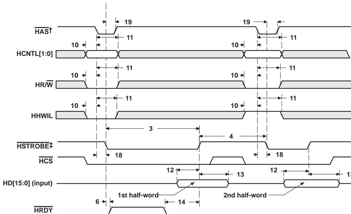
† For correct operation, strobe the  $\overline{\text{HAS}}$  signal only once per  $\text{HSTROBE}$  active cycle.
