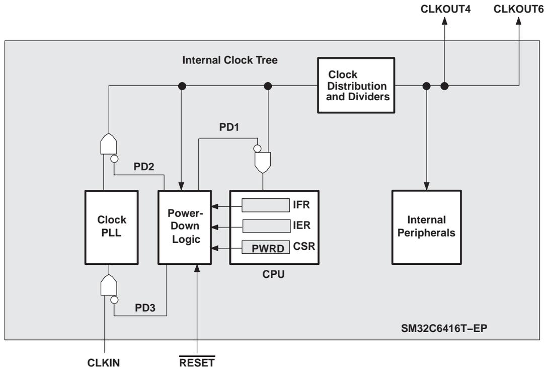
† External input clocks, with the exception of CLKIN, are *not* gated by the power-down mode logic.
