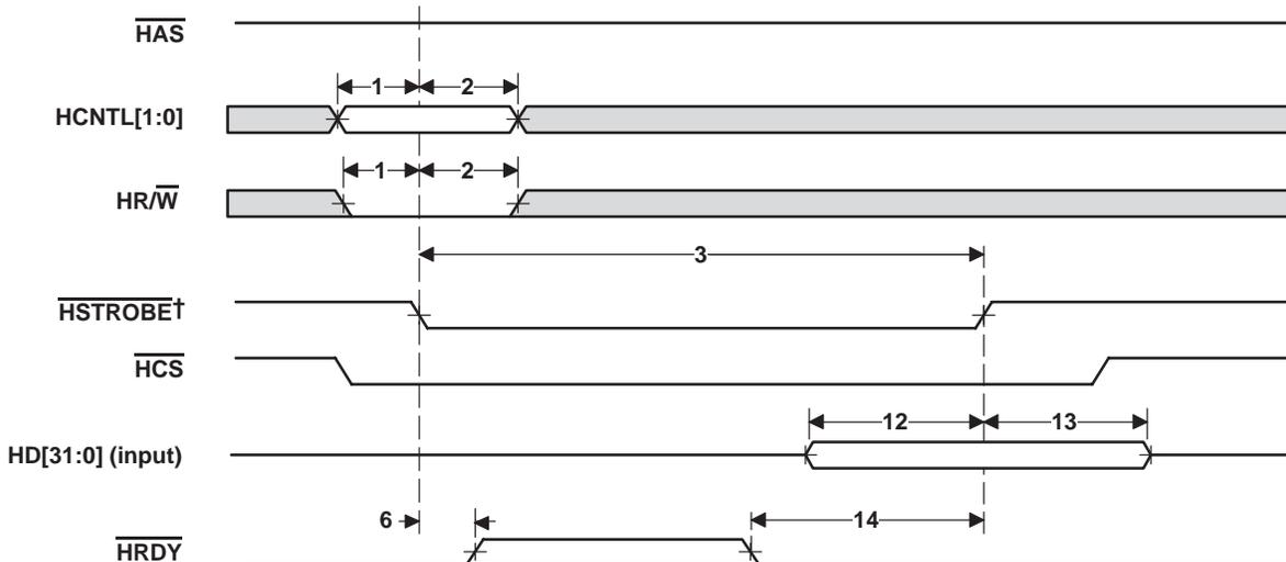
†  $\overline{\text{HSTROBE}}$  refers to the following logical operation on  $\overline{\text{HCS}}$ ,  $\overline{\text{HDS1}}$ , and  $\overline{\text{HDS2}}$ :  $[\text{NOT}(\overline{\text{HDS1}} \text{ XOR } \overline{\text{HDS2}})] \text{ OR } \overline{\text{HCS}}$ .
