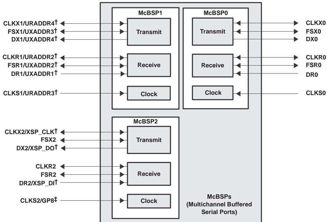
† These McBSP2 and McBSP1 pins are MUXed with the PCI and UTOPIA peripherals, respectively. By default, these signals function as McBSP2 and McBSP1, respectively. For more details on these MUXed pins, see the Device Configurations section of this data sheet.
