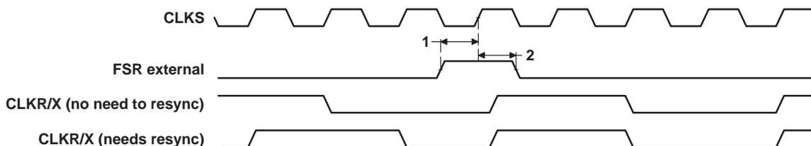
Figure 52. FSR Timing When GSYNC = 1
