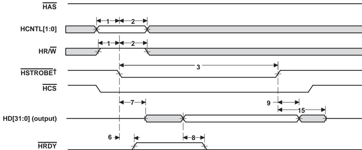
$^\dagger$   $\overline{\text{HSTROBE}}$  refers to the following logical operation on  $\overline{\text{HCS}}$ ,  $\overline{\text{HDS1}}$ , and  $\overline{\text{HDS2}}$ :  $[\text{NOT}(\overline{\text{HDS1}} \text{ XOR } \overline{\text{HDS2}})] \text{ OR } \overline{\text{HCS}}$ .
