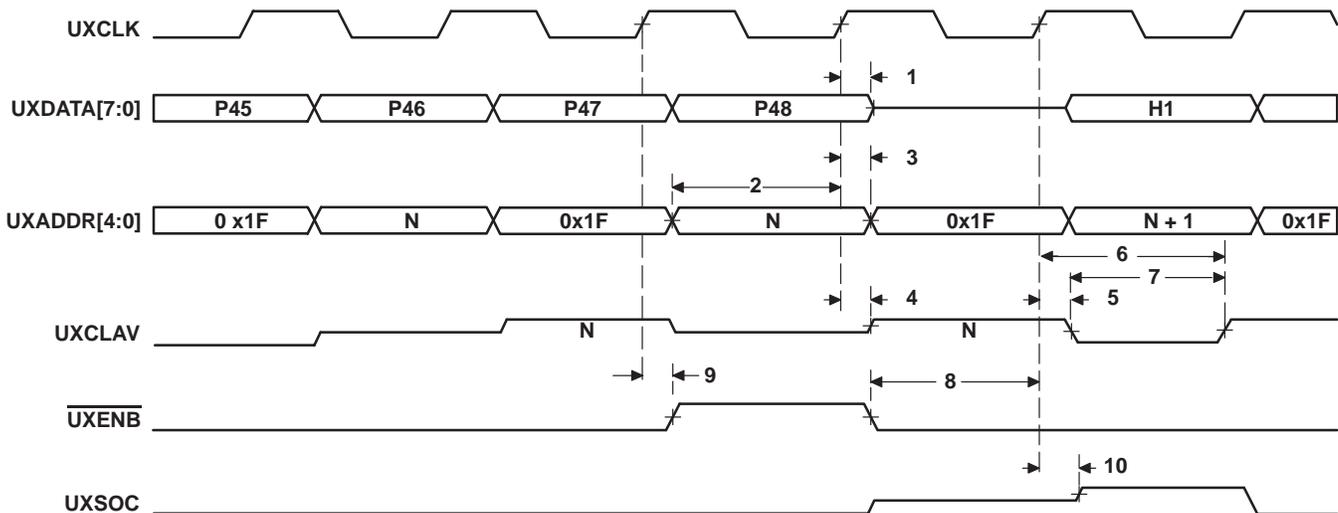
† The UTOPIA Slave module has signals that are middle-level signals indicating a high-impedance state (i.e., the UXCLAV and UXSOC signals).
