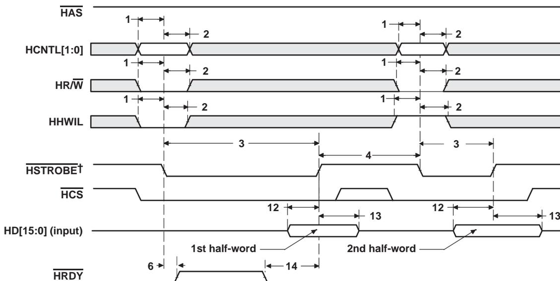
†  $\text{HSTROBE}$  refers to the following logical operation on  $\overline{\text{HCS}}$ ,  $\overline{\text{HDS1}}$ , and  $\overline{\text{HDS2}}$ :  $[\text{NOT}(\overline{\text{HDS1}} \text{ XOR } \overline{\text{HDS2}})] \text{ OR } \overline{\text{HCS}}$ .
