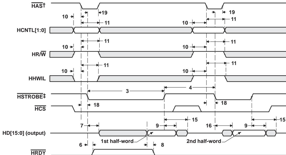
† For correct operation, strobe the  $\overline{\text{HAS}}$  signal only once per  $\text{HSTROBE}$  active cycle.
