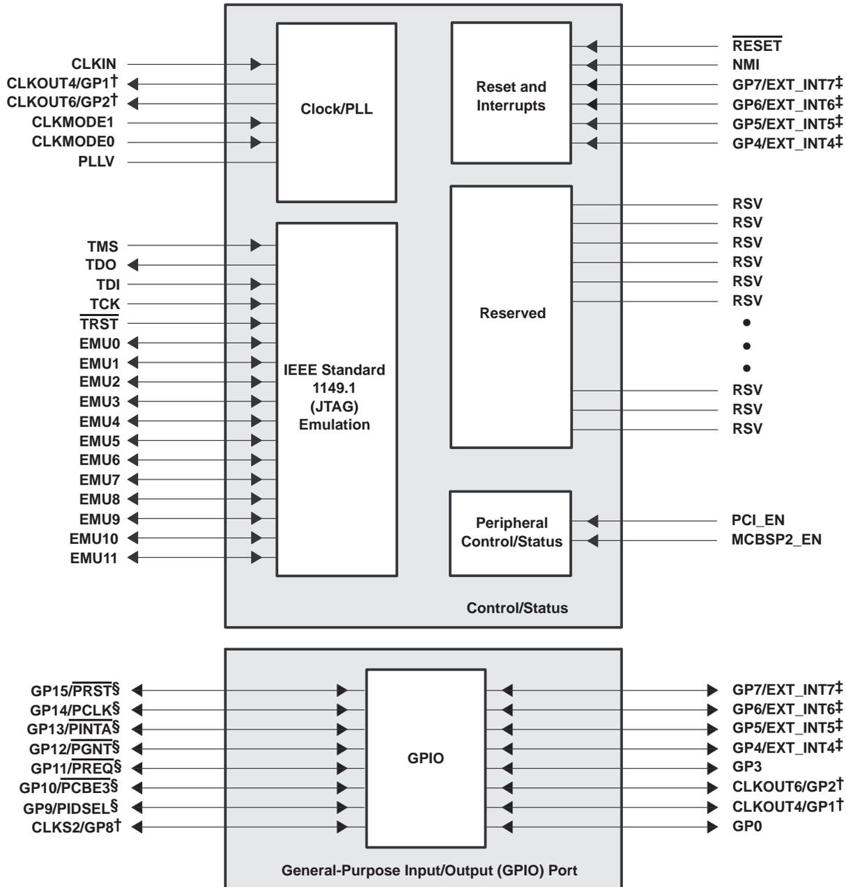
† These pins are MUXed with the GPIO port pins and by default these signals function as clocks (CLKOUT4 or CLKOUT6) or McBSP2 clock source (CLKS2). To use these MUXed pins as GPIO signals, the appropriate GPIO register bits (GPxEN and GPxDIR) must be properly enabled and configured. For more details, see the Device Configurations section of this data sheet.
