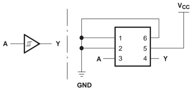
Figure 11. 17/34: Noninverted Buffer
