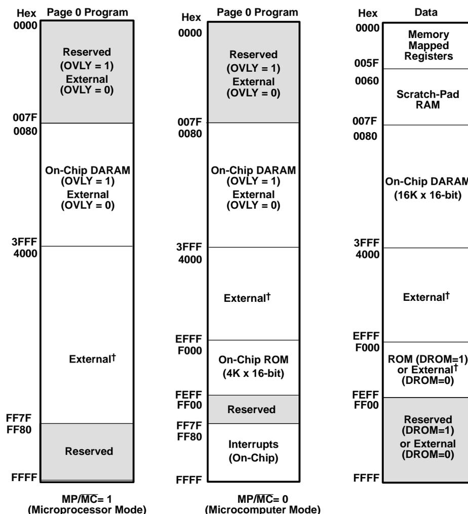
† Only six of the 16 total TMS320UC5405 address bits are available to the external interface; therefore, only 64 unique external addresses are available, regardless of the actual 16-bit address generated internally. These 64 addresses are those resulting from the truncation of the upper address bits (A6 and above). This results in these 64 addresses being repeated throughout all of the external address space.
