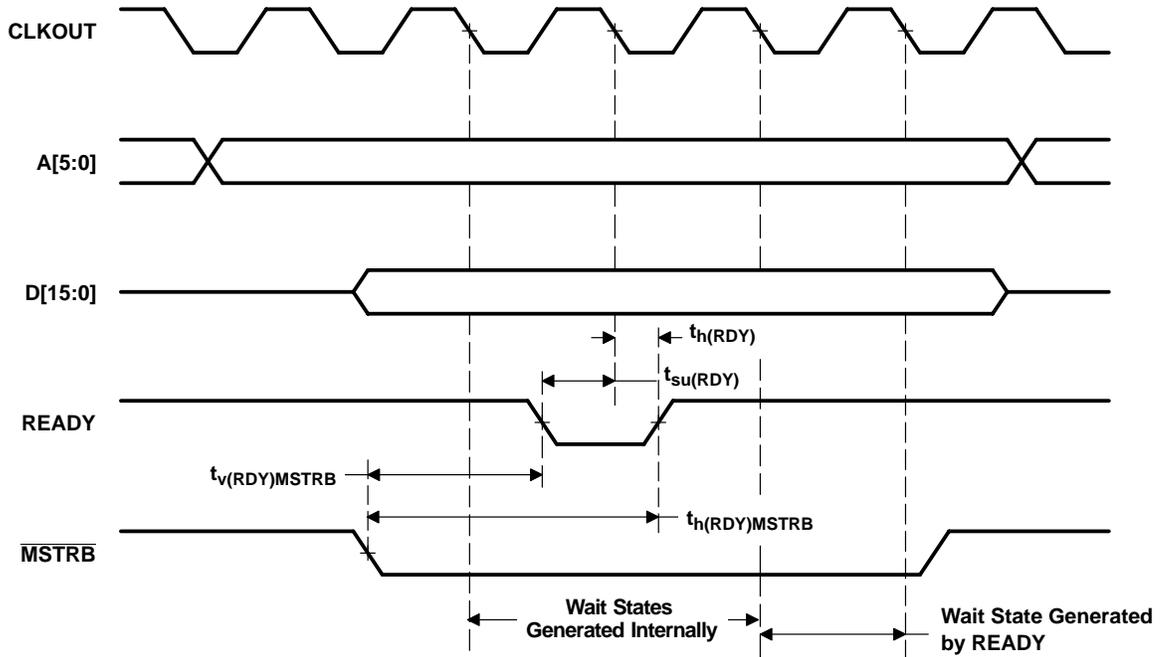
Figure 6–10. Memory Write With Externally Generated Wait States
