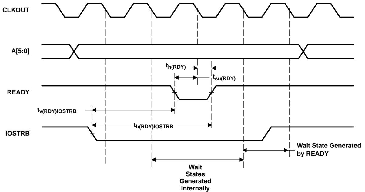
Figure 6–11. I/O Read With Externally Generated Wait States
