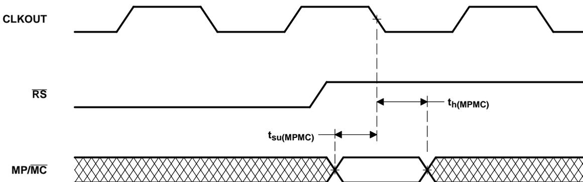
Figure 6-16. MP/MC Timing
