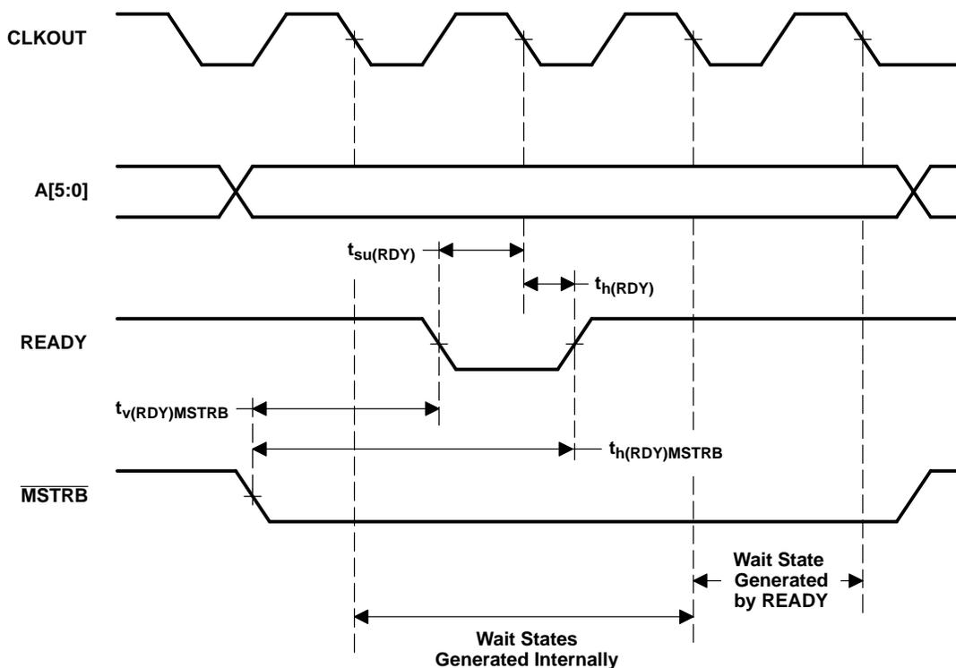
**Figure 6–9. Memory Read With Externally Generated Wait States**
