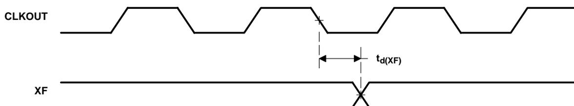
**Figure 6–18. XF Timing**
