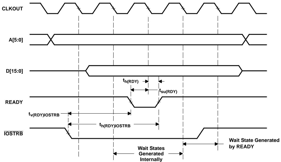
Figure 6-12. I/O Write With Externally Generated Wait States
