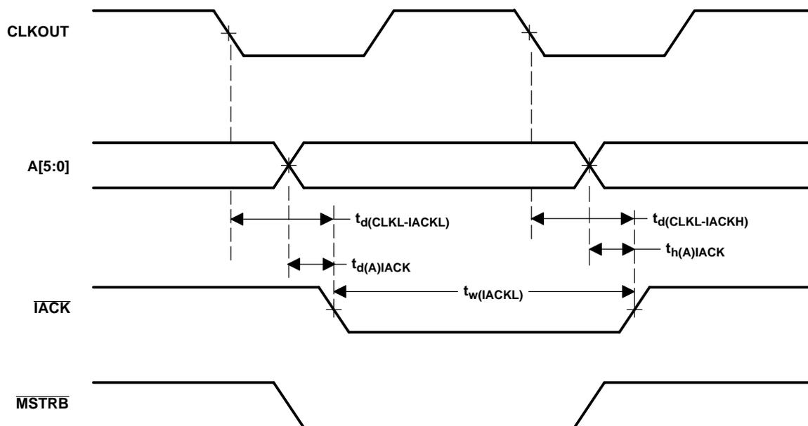
**Figure 6–17.  $\overline{\text{IACK}}$  Timings**
