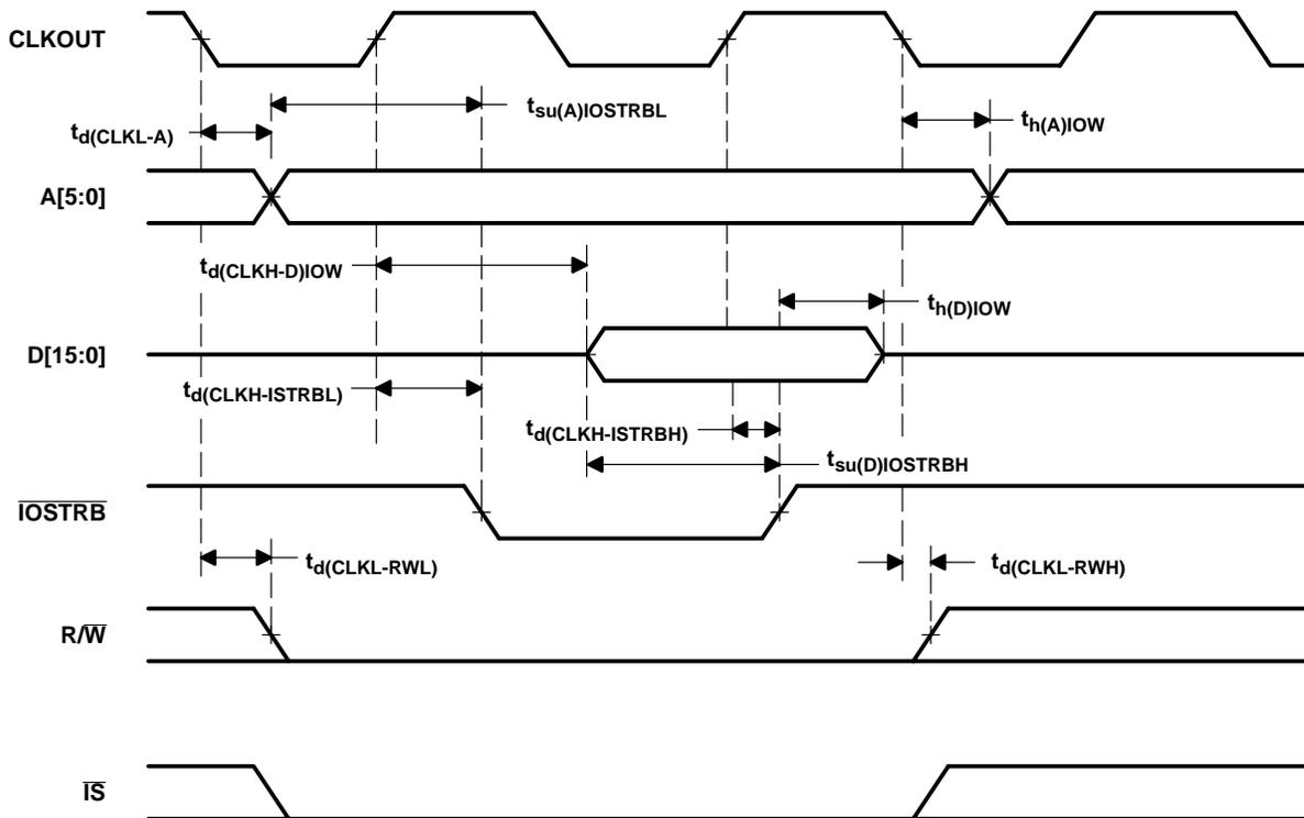
**Figure 6–8. Parallel I/O Port Write**
