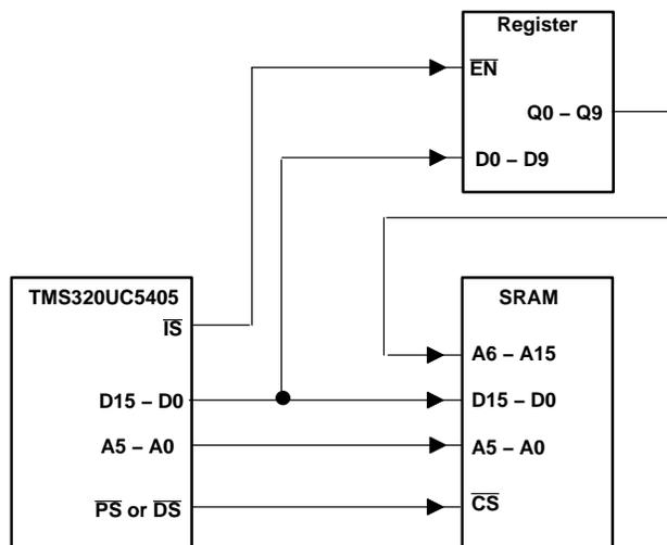
Figure 3-3. TMS320UC5405 External Memory Paging Scheme
