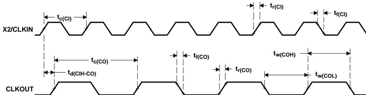
**Figure 6–3. External Divide-by-Two Clock Timing**
