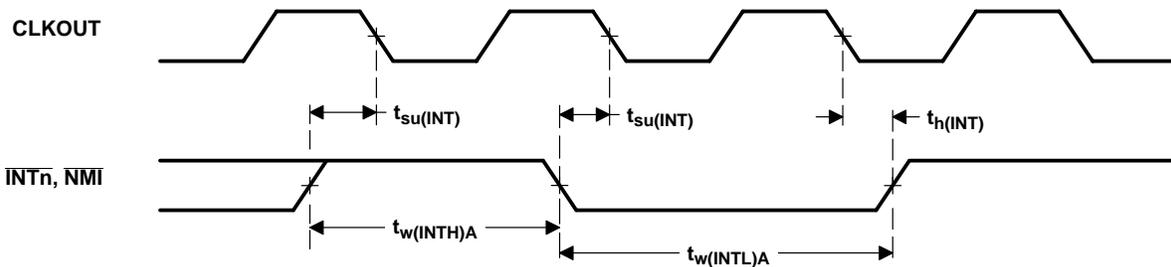
Figure 6-15. Interrupt Timing
