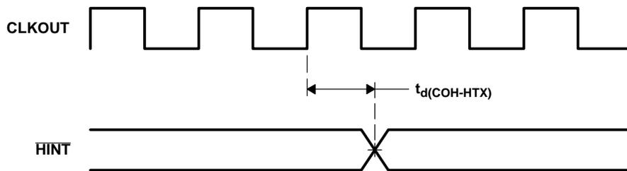
Figure 6-29.  $\overline{\text{HINT}}$  Timing
