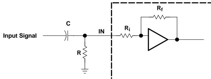
**Figure 35. Resistor on Input for Cut-Off Frequency**
