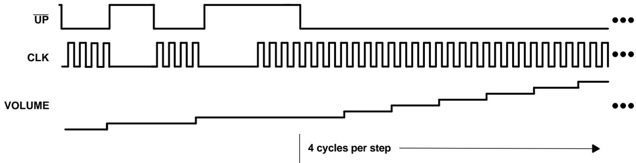
Figure 33. External Clock (4 Cycles Per Volume Change)
