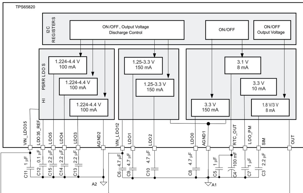
Figure 39. Required External Components, Recommended Values, External Connections
