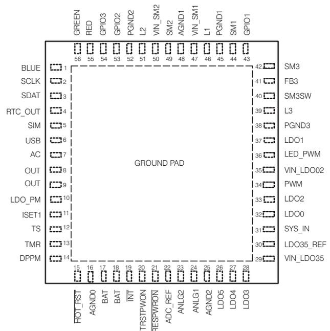
QFN 56-Pin, 7 x 7 mm Package
