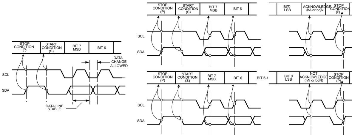
Figure 24. I<sup>2</sup>C operation waveforms
