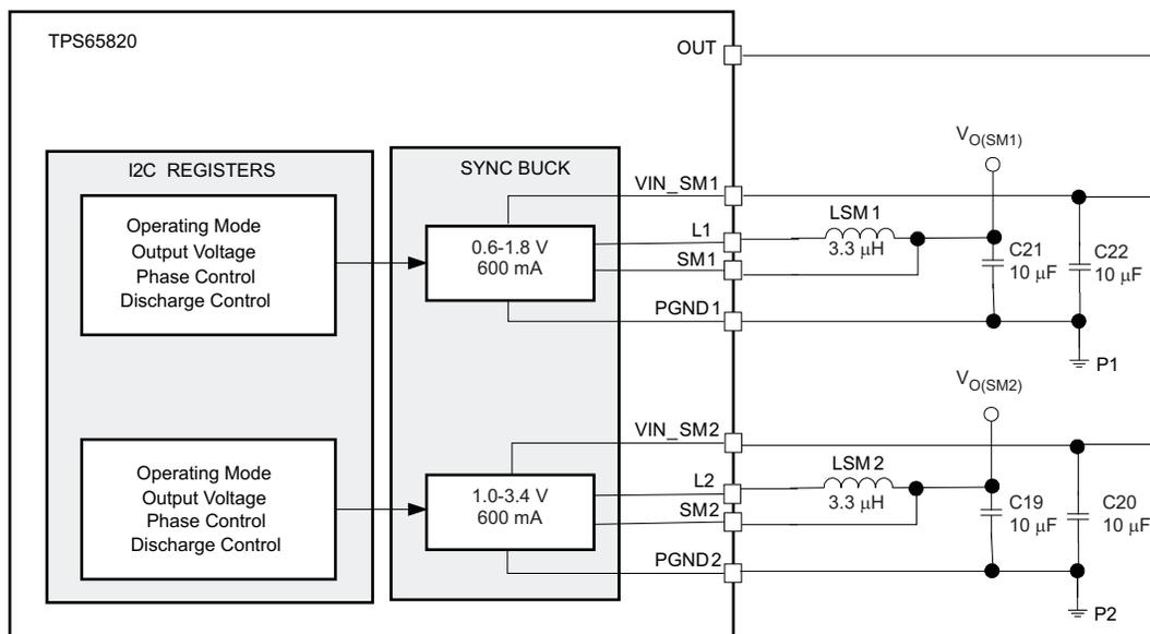
Figure 41. Required External Components, Recommended Values, External Connections
