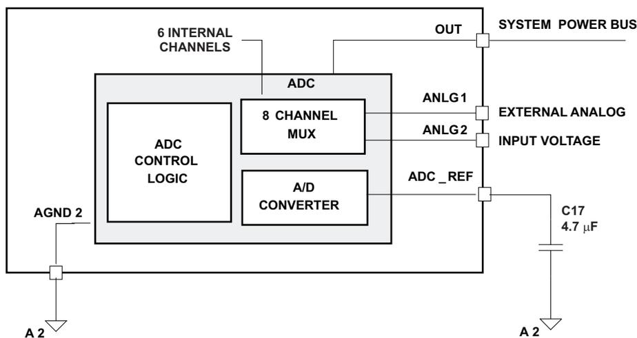
Figure 47. Required External Components, Recommended Values, External Connections
