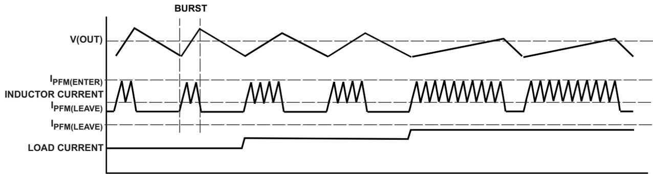
**Figure 46. Typical Burst Operation in PFM Mode**
