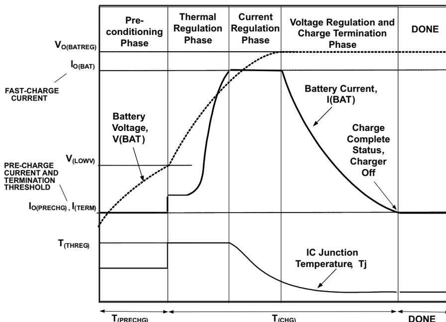
Figure 36. Typical Charge Cycle, Thermal Loop Active
