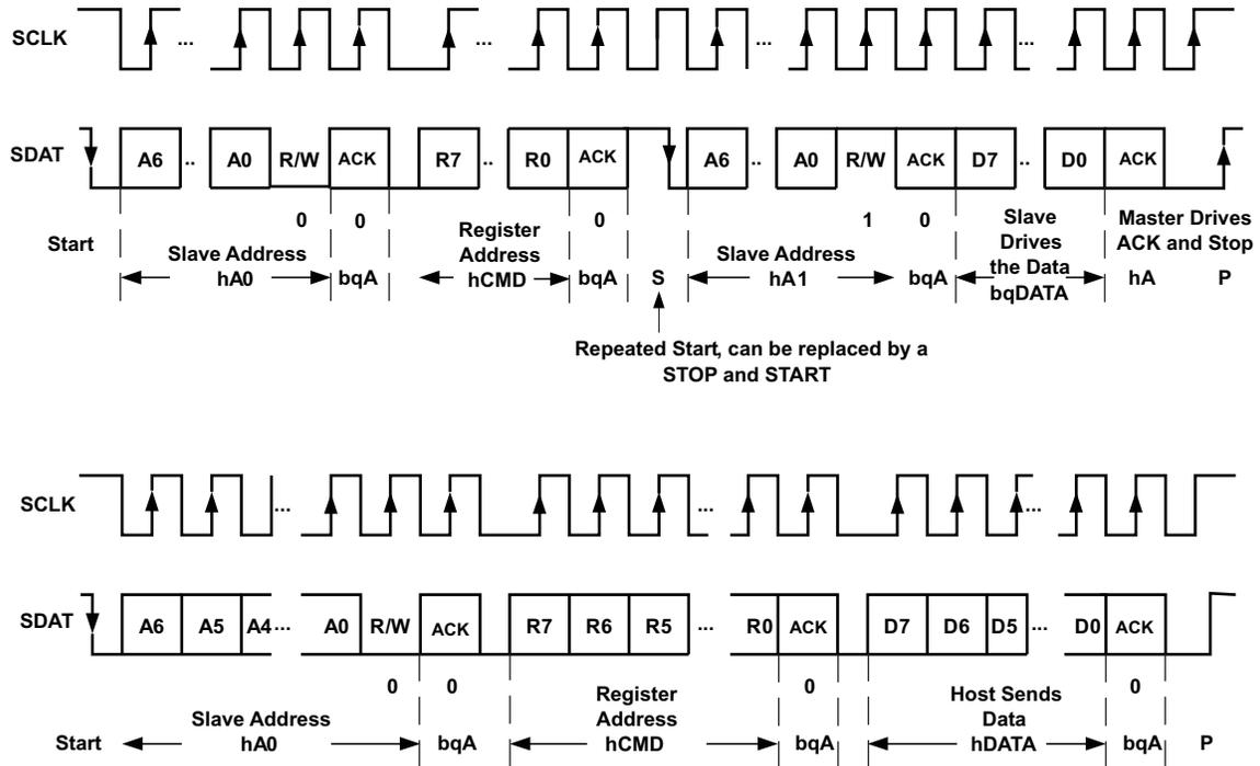
Figure 25. I<sup>2</sup>C read and write operations
