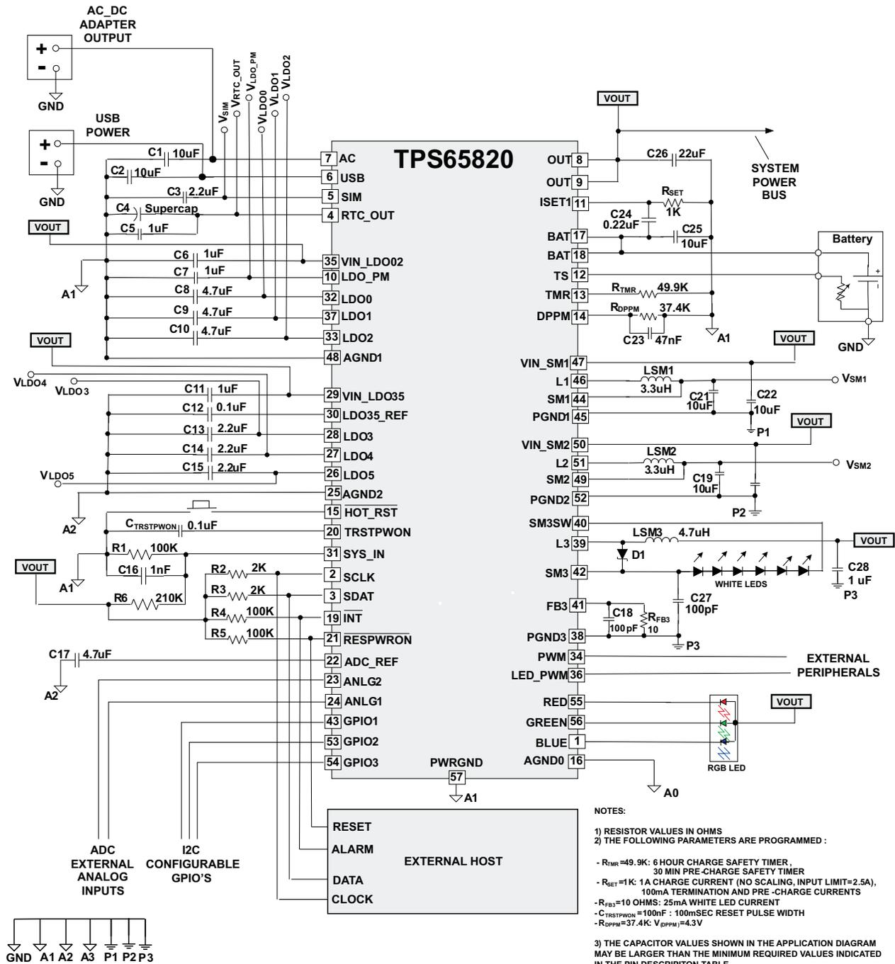
Figure 3. TPS65820 Application Diagram, Recommended External Components
