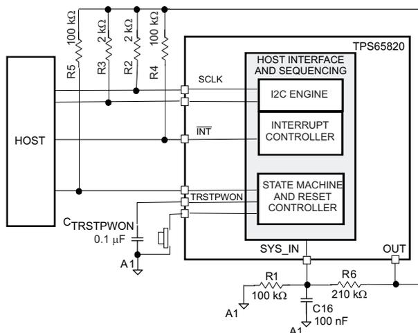
Figure 26. Required External Components, Recommended Values, External Connections
