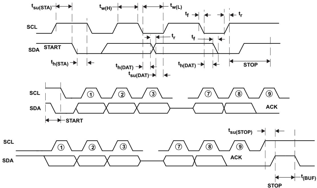
Figure 2. I<sup>2</sup>C Timing
