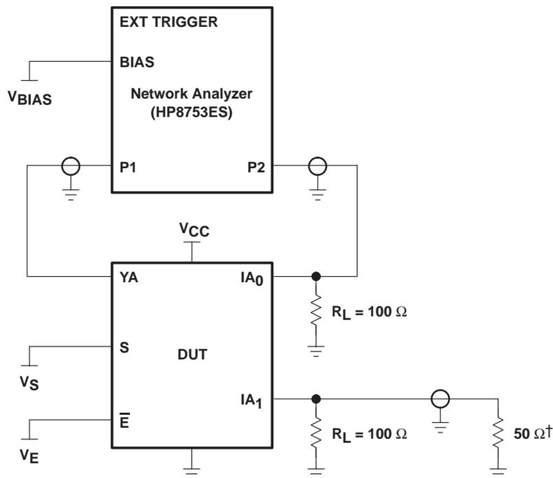
† A 50-Ω termination resistor is needed for the network analyzer.
