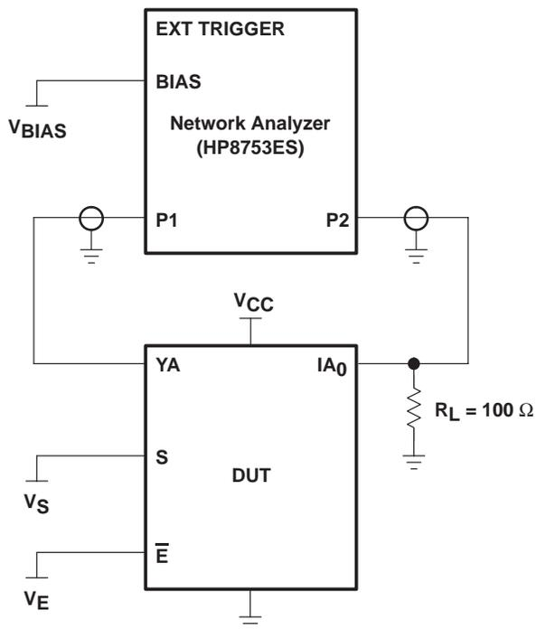
Figure 5. Test Circuit for Frequency Response (BW)
