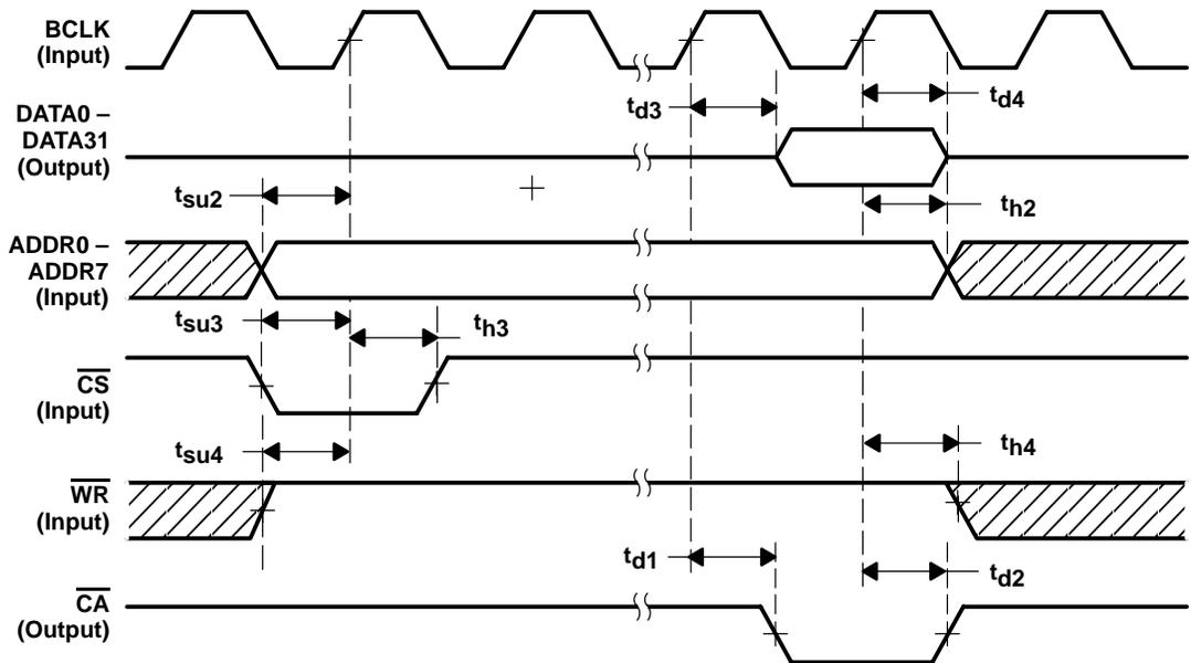
NOTE A. Following a  $\overline{CS}$  assertion, there may be a maximum of 9 rising edges of BCLK before a  $\overline{CA}$  is returned.  $\overline{CA}$  must be returned before another  $\overline{CS}$  may be asserted.
