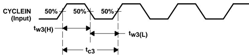
Figure 6-13. CYCLEIN Waveform
