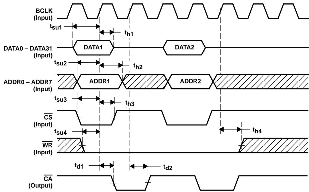
NOTE A. There must be a minimum of 3 rising edges of BCLK between assertions of  $\overline{CS}$ .
