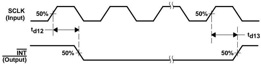
Figure 6-12. Interrupt Waveform
