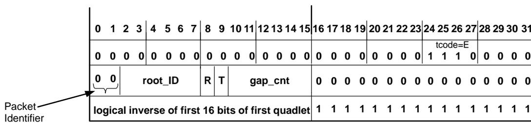
Figure 4–21. PHY-Configuration Packet Format
