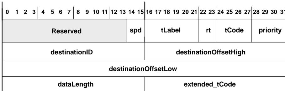
Figure 4–6. Block-Transmit Format (Read Request)
