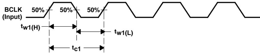
Figure 6-1. BCLK Waveform
