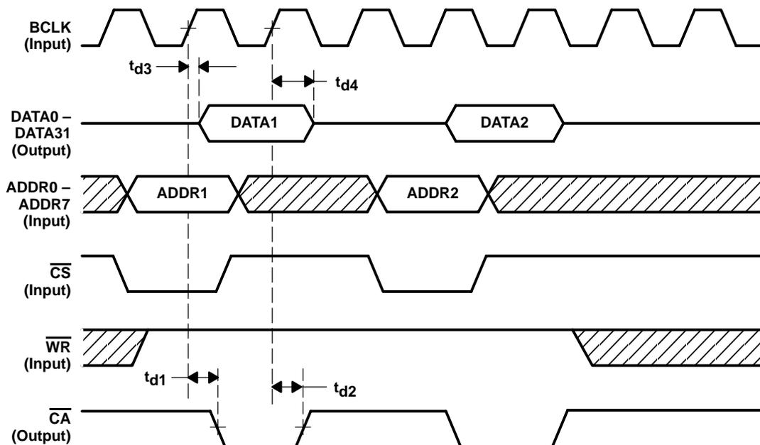
NOTE A. There must be a minimum of 3 edges of BCLK between assertions of  $\overline{CS}$ .
