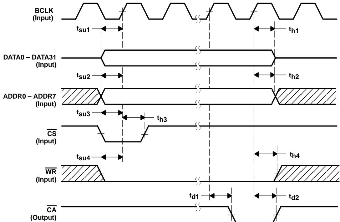
NOTE A. Following a  $\overline{CS}$  assertion, there may be a maximum of 9 rising edges of BCLK before a  $\overline{CA}$  is returned.  $\overline{CA}$  must be returned before another  $\overline{CS}$  may be asserted.
