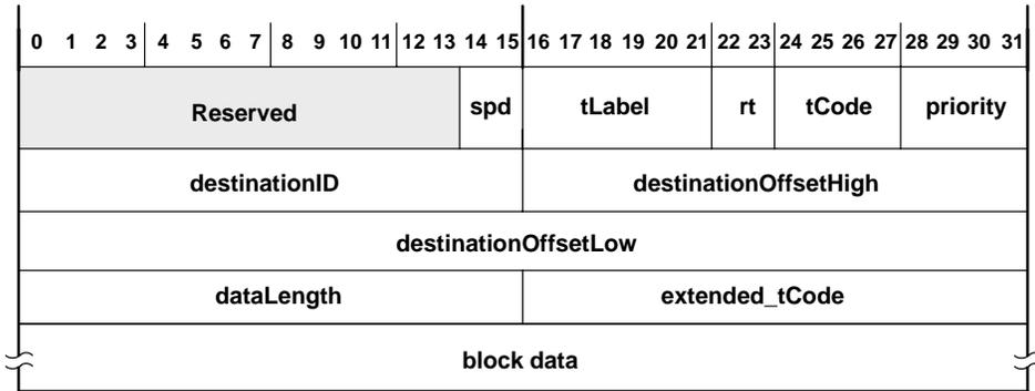
Figure 4–5. Block-Transmit Format (Write Request)
