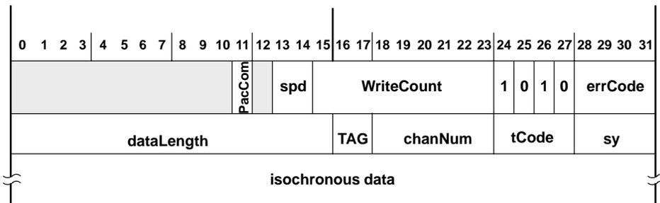
Figure 4–18. Isochronous-Receive Format
