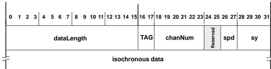
Figure 4–17. Isochronous-Transmit Format
