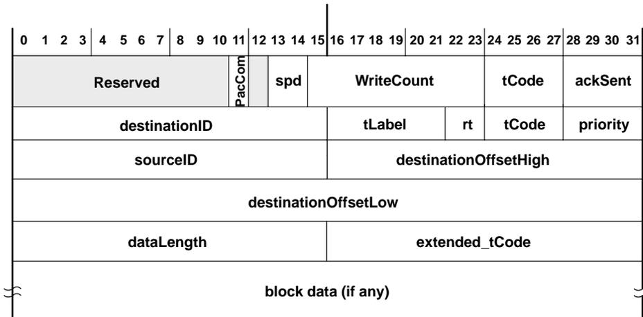
Figure 4–13. Block-Receive Format (Write Request)
