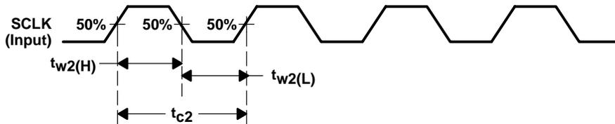
Figure 6–8. SCLK Waveform
