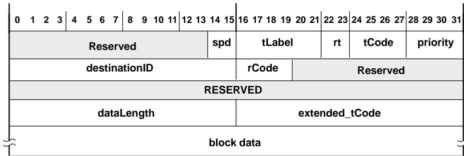
Figure 4–8. Block-Transmit Format (Write Response)
