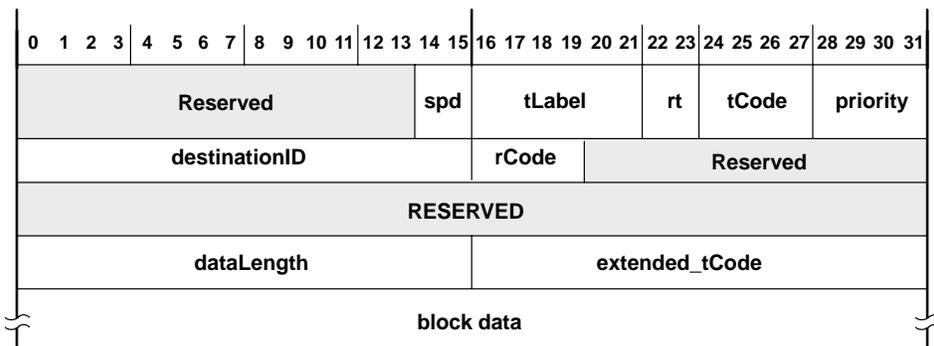
Figure 4–7. Block-Transmit Format (Read Response)
