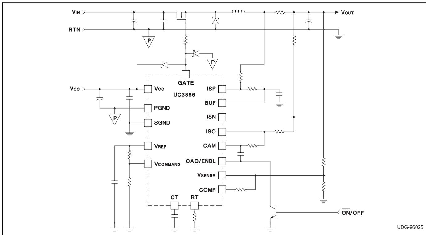
Figure 7. The UC3886 Configured in a Buck Regulator
