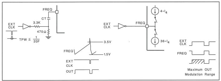
Figure 4. External clock synchronization.
