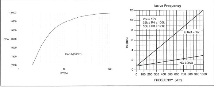
Figure 5. Frequency dependence on RT/R4 ratio.
