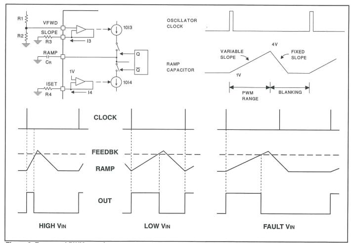
Figure 2. Ramp and PWM waveforms.
