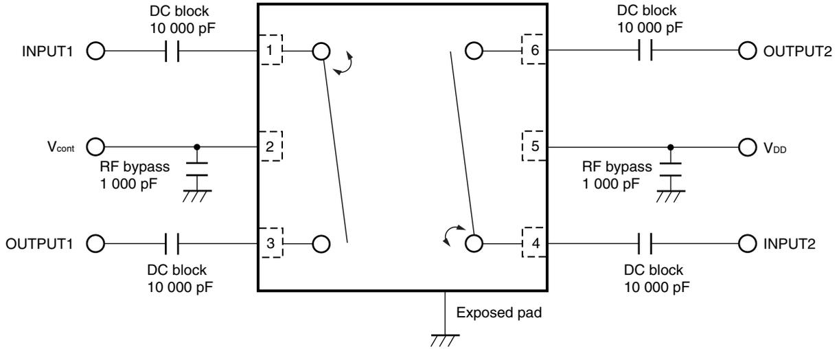
**Caution** This IC has pull down resistances inside between each RF line and GND line, which bias each RF pin internally to GND, then the IC cannot be used for DC switching.
