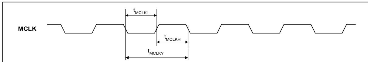
Figure 4 Master Clock Timing Requirements
