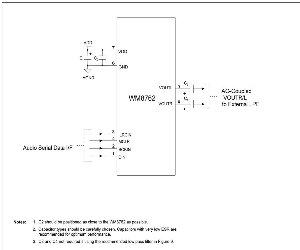
Figure 13 External Component Diagram
