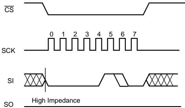
FIGURE 5. WRITE ENABLE/DISABLE LATCH SEQUENCE (WREN/WRDI INSTRUCTION)
