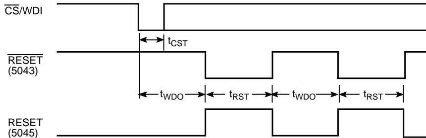
**RESET/RESET Output Timing**
