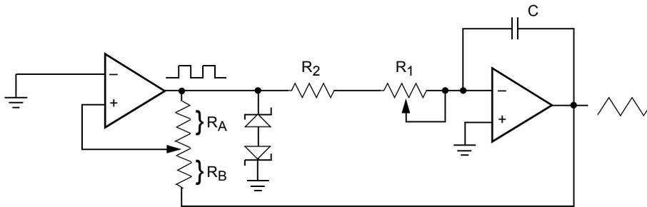
$$\text{Frequency} \propto R_1, R_2, C$$
