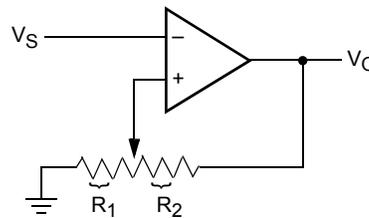
$$V_{UL} = \{R_1/(R_1 + R_2)\} V_O(\text{max})$$
