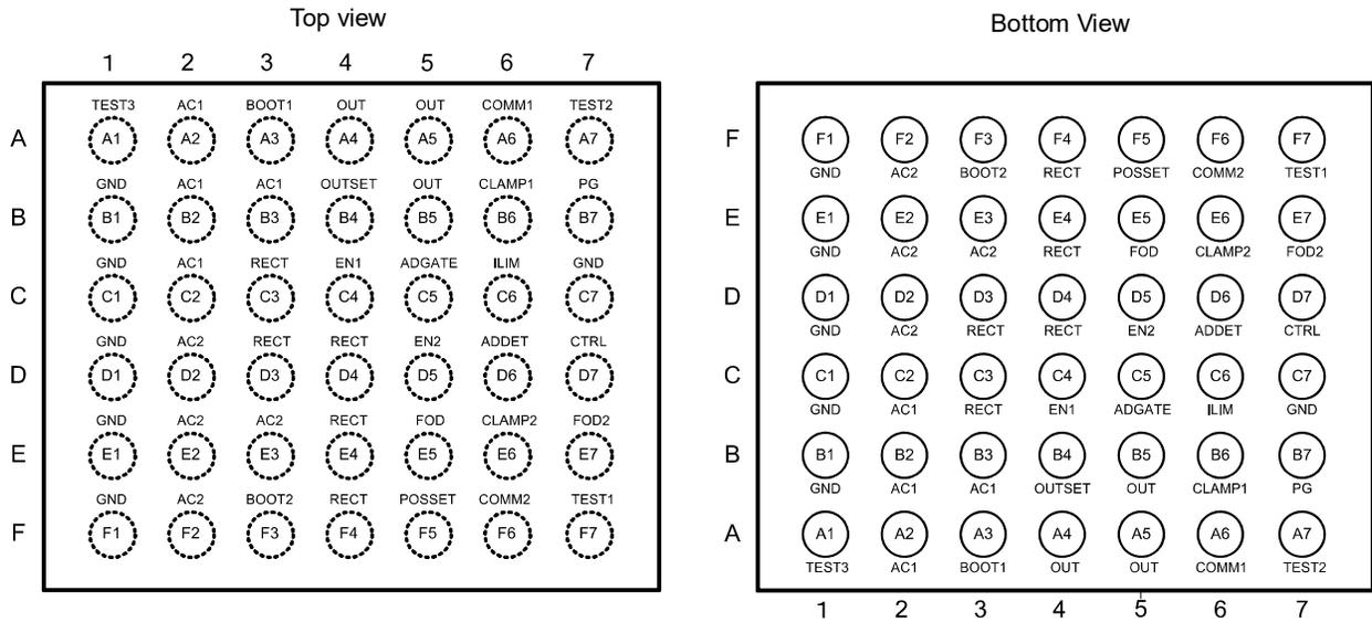
Figure 7. Pin configuration
