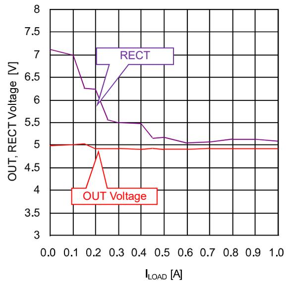
Figure 4. OUT Voltage [V] and RECT Voltage [V] vs. I<sub>LOAD</sub> [A] (R<sub>SET</sub>=27k Ω)
