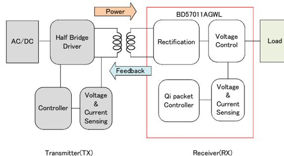
Figure 2. Product position in Wireless Power Supply System
