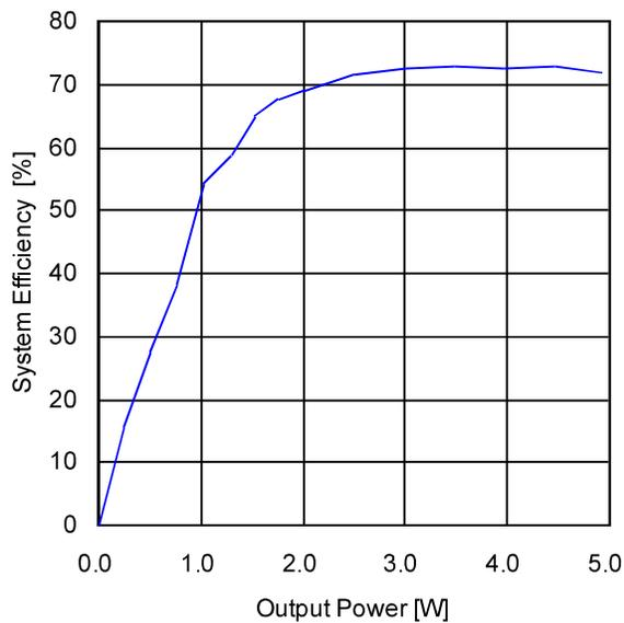
Figure 5. System Efficiency [%] vs. Output Power [W] (R<sub>SET</sub>=27k Ω)
