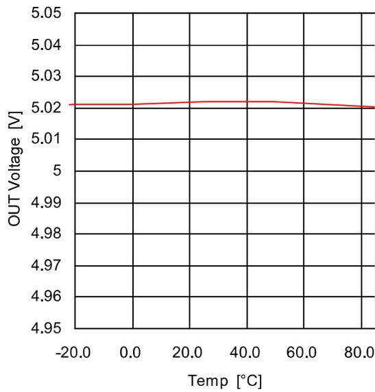
Figure 3. OUT Voltage [V] vs. Temp. [°C] (R<sub>SET</sub>=27k Ω)
