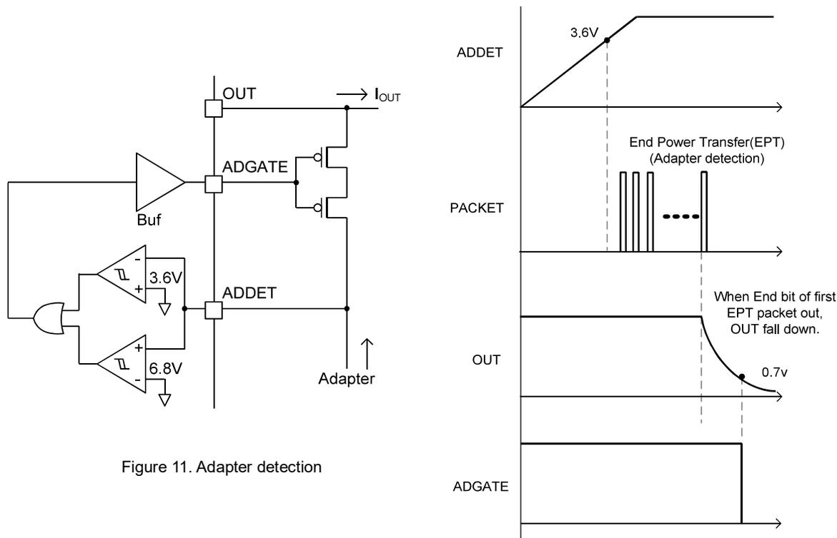
Figure 11. Adapter detection
