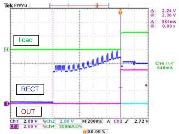
Figure 6. Startup Waveform (R<sub>SET</sub>=27k Ω)
