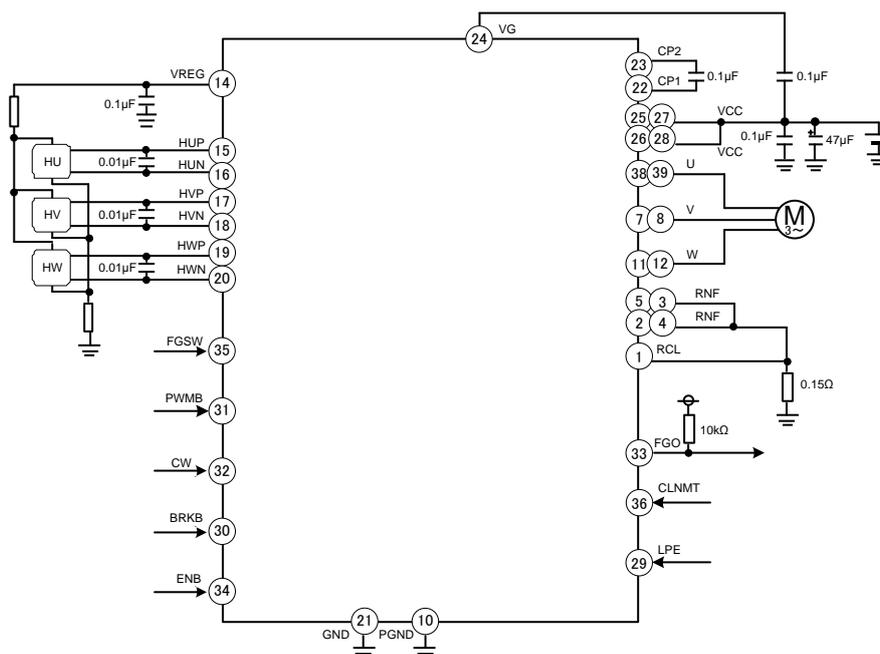
Figure 1. Application Circuit
