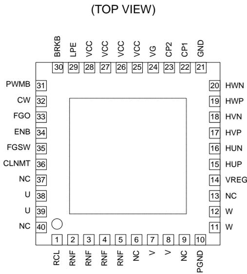
Figure 2. Pin Configuration
