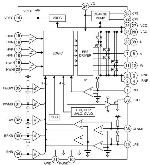
Figure 3. Block Diagram
