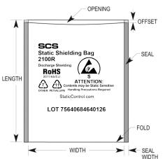
Tolerance: Width -0, +1/4" Length ± 1/8" Offset 0 to 1/4" Seal width 3/8" with a tolerance of ± 1/8"
