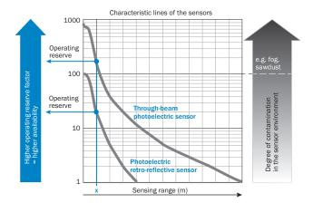
At a sensing range of "x" the photoelectric retro-reflective and through-beam photoelectric sensors have different operating reserves (see blue arrow). The higher the operating reserve factor, the better the sensor can compensate the contamination in the air or in the light beam and on the optical surfaces (front screen, reflector), i.e. the sensor has the maximum availability, otherwise the sensor switches due to pollution although there is no object in the path of the light beam.
