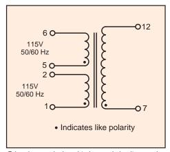
Primaries are designed to be used simultaneously. That is, they must be used either series or parallel connected (as one winding).
