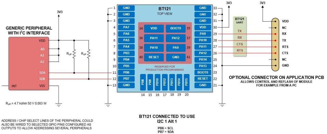
**Figure 20 Connecting to an I<sup>2</sup>C peripheral**
