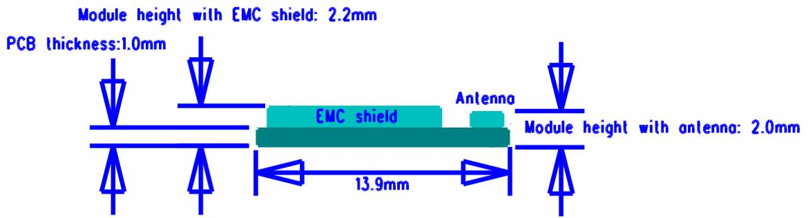
Figure 23 BT121 module side view dimensions
