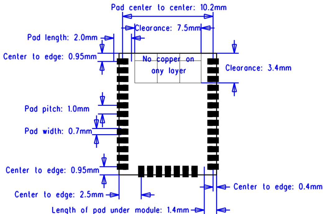
Figure 22 BT121 module recommended PCB pad pattern
