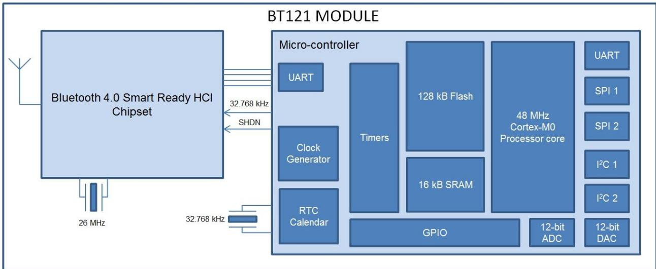
**Figure 1 BT121 Bluetooth Smart Ready module block diagram**
