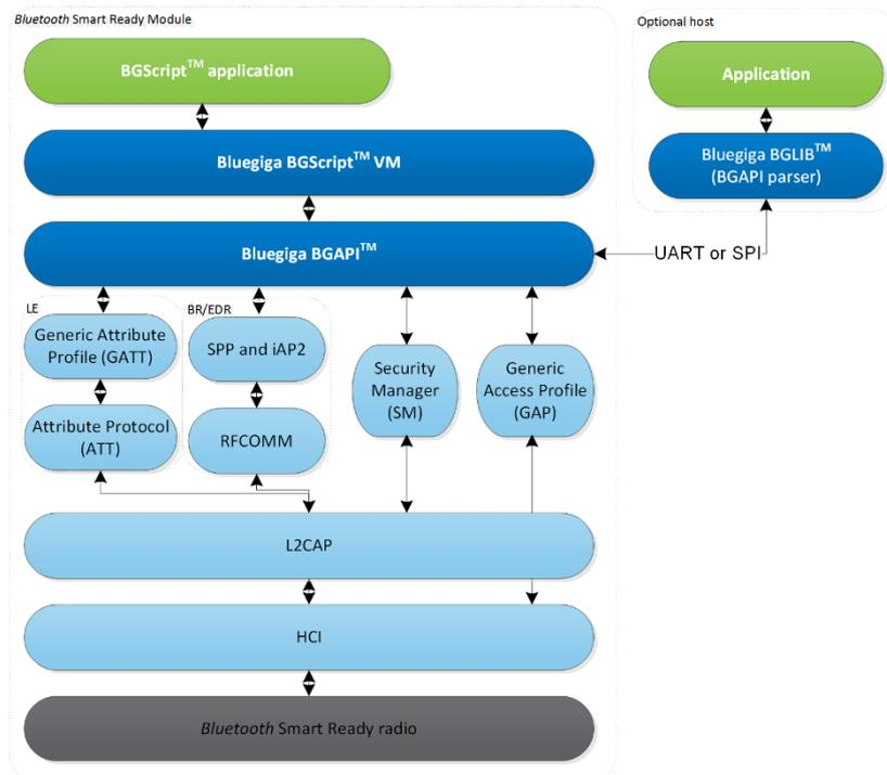
Figure 17 Bluegiga Bluetooth Smart Ready software stack
