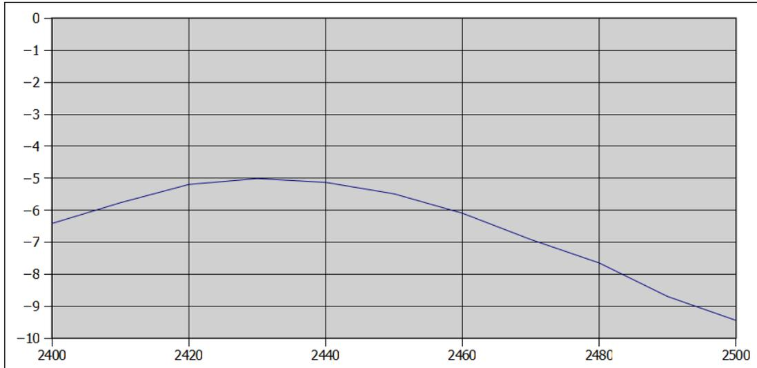
**Figure 11** Antenna efficiency related to frequency
