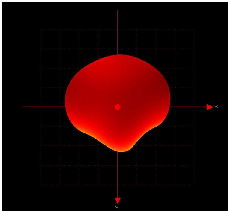
Figure 16 Typical 3D radiation pattern for BT121 with view from above the module
