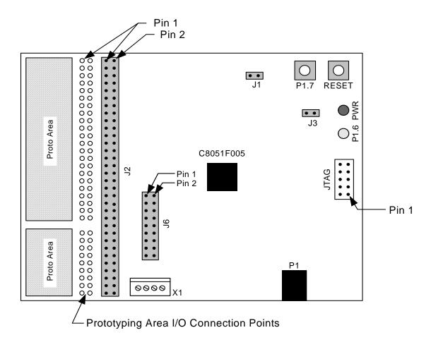
Figure 2. C8051F005 Target Board
