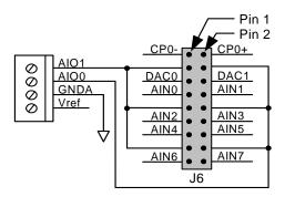
Figure 3. J6 Analog I/O Configuration Connector
