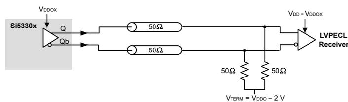
Figure 2.8. LVPECL AC and DC Output Terminations
