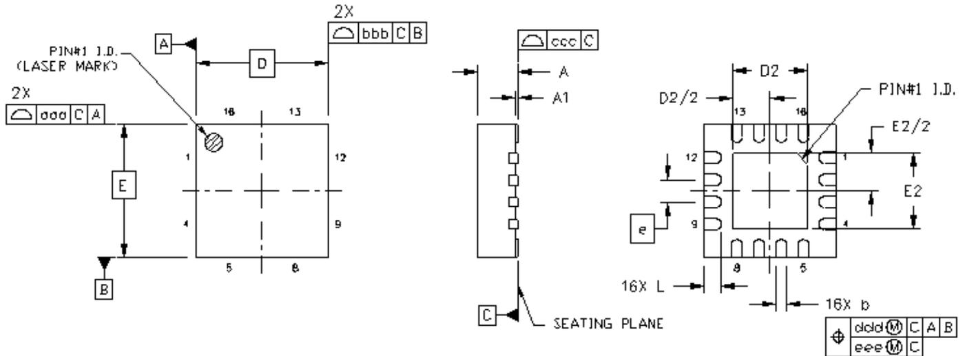
Figure 6.1. 3x3 mm 16-QFN Package Diagram Dimensions
