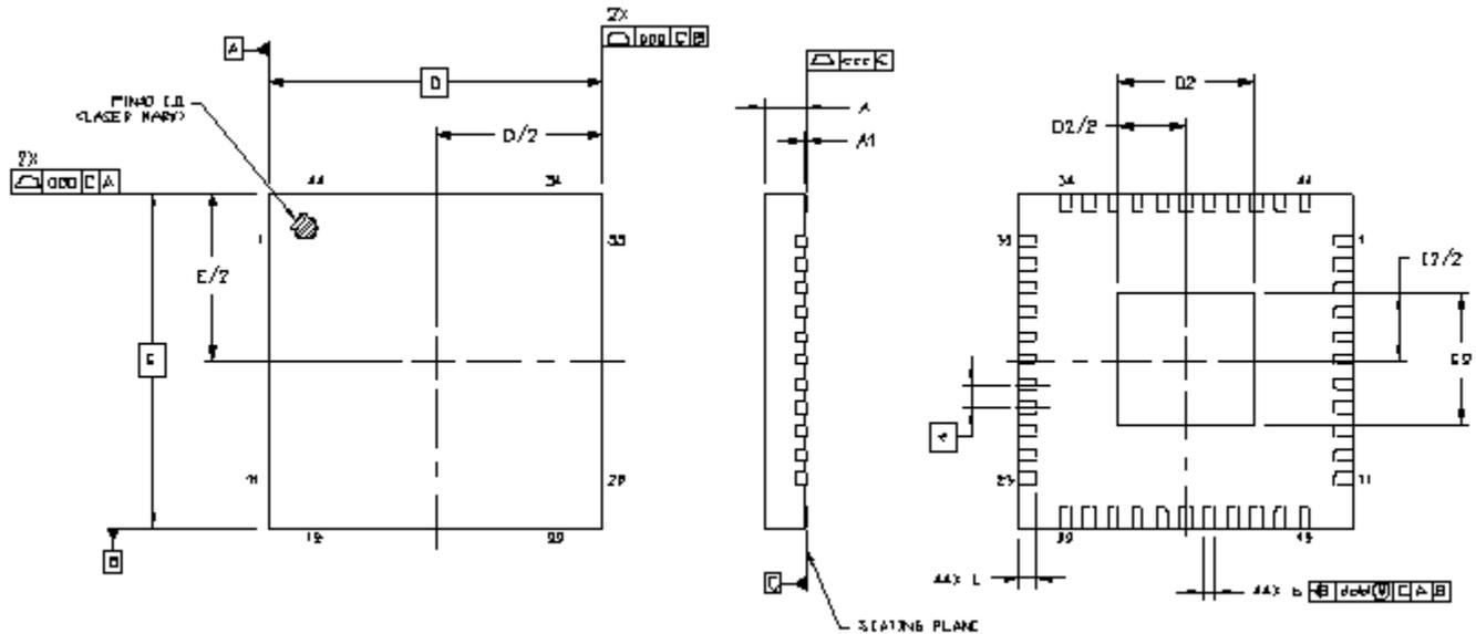
Figure 6.3. 7x7 mm 44-QFN Package Diagram Dimensions
