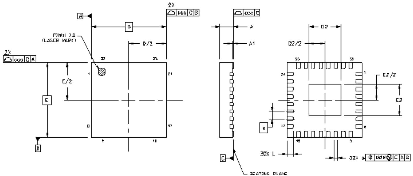
Figure 6.2. 5x5 mm 32-QFN Package Diagram Dimensions
