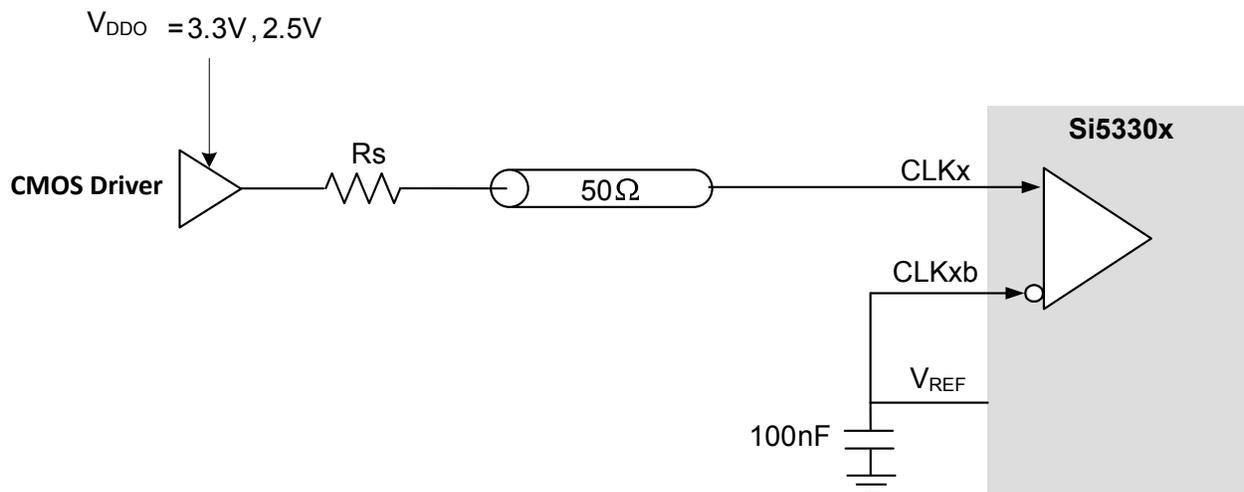
Figure 2.6. Using Voltage Reference with Single-Ended Input Clock
