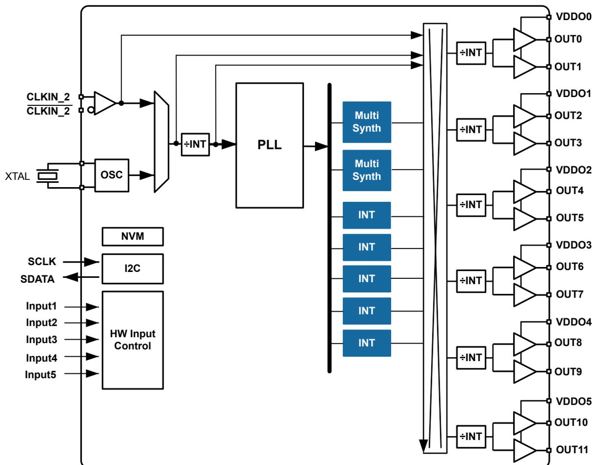
Figure 3.1. Block Diagram for 12-Output Si5357 in 32-QFN
