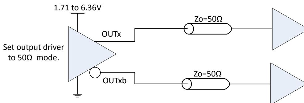
Figure 3.3. LVCMOS Output Termination Example, Option 1
