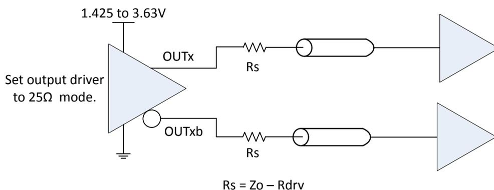
Figure 3.4. LVCMOS Output Termination Example, Option 2
