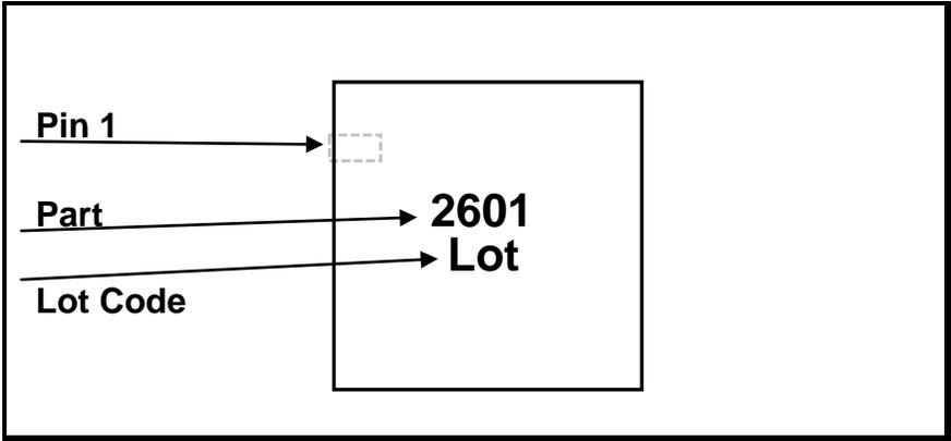
**Figure 4: SE2601T Branding and Pin 1 Location**
