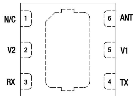
**Figure 2. SKY13446-374LF Pinout – 6-Pin MLPD (Top View)**
