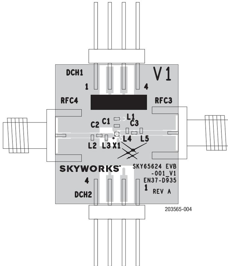
Figure 4. SKY65623-682LF Evaluation Board Assembly Diagram
