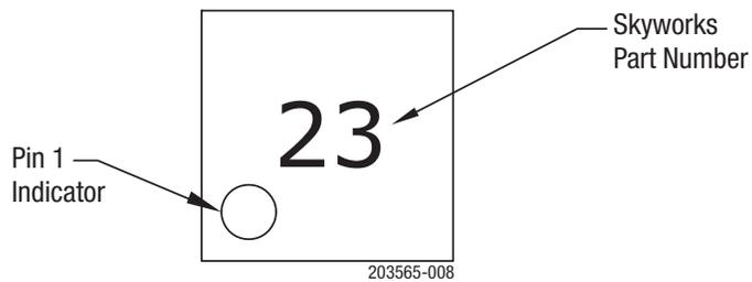
**Figure 8. SKY65623-682LF Typical Part Marking (Top View)**
