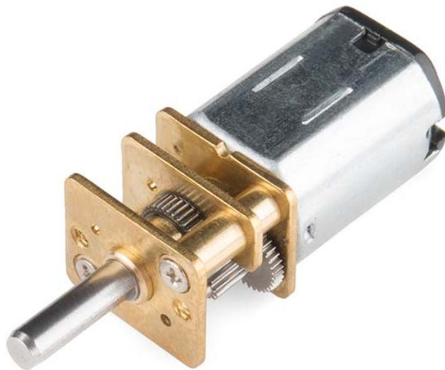
These micro gearmotors are incredibly tough and feature full metal gears. They have a gear ratio of 30:1 and operate up to 12 volts and have a stall torque of 9 oz-in. and a max speed of 900 RPM. Each micro gearmotor sports a 3mm D-shaft.
