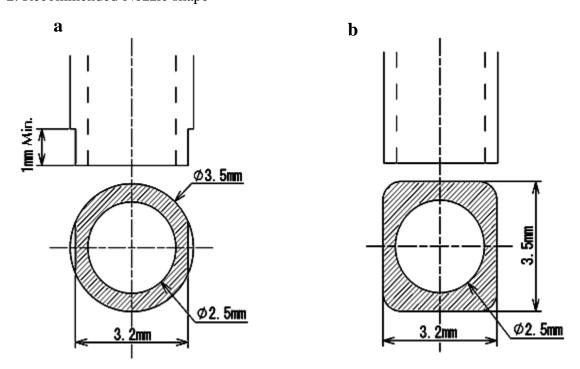
\*Nozzle with chamfering is recommended
