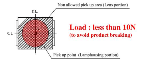
Please adjust the load, the pick up point, the nozzle diameter, etc. before mounting because the over load can cause the breakage of the lamp housing.
