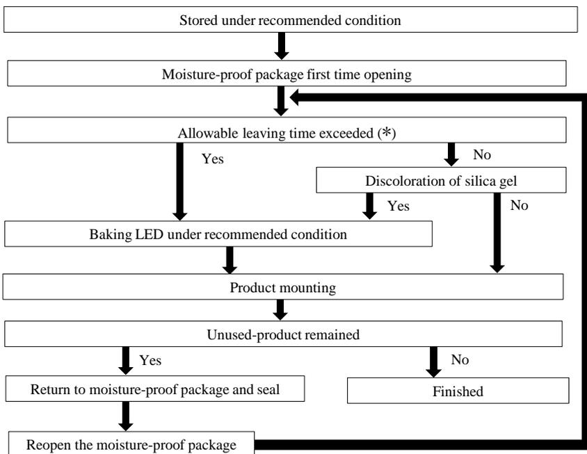
Allowable leaving time means the maximum allowable leaving time after opening package, which depends on each LED type. The allowable leaving time should be calculated from the first opening of package to the time when soldering process is finished. When judging if the allowable leaving time has exceeded or not, please subtract the soldering time. The allowable leaving time after reopening should be calculated from the first opening of package, or from the time when baking process is finished.
