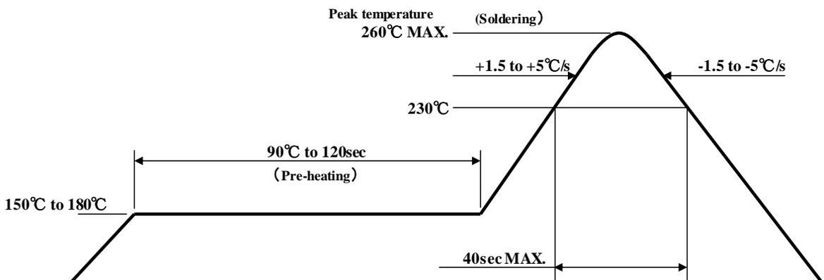
Notes 1 Temperature Profile for the reflow should be set to the surface temperature of resin which is on the top of LED. This should be the maximum temperature for soldering. Lowering the heating temperature and decreasing heating time is very effective in achieving higher reliability.
