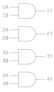
FIGURE 3. Logic diagram.
