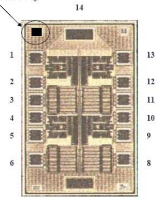
Pad size: Pad numbers 1 to 6 and 8 to 13: 100 x 100  $\mu$ m Pad numbers 7 (GND) and 14 (V<sub>CC</sub>): 100 x 280  $\mu$ m
