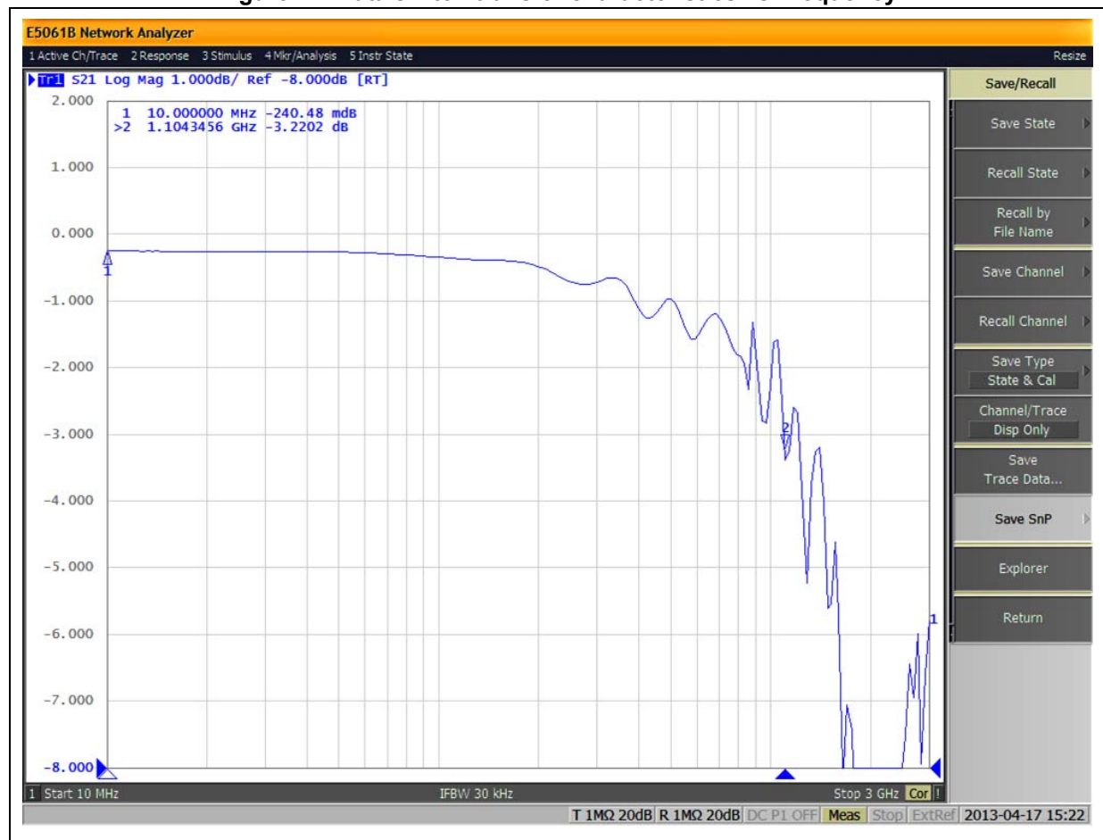
Figure 17. Data switch transfer characteristics vs. frequency
