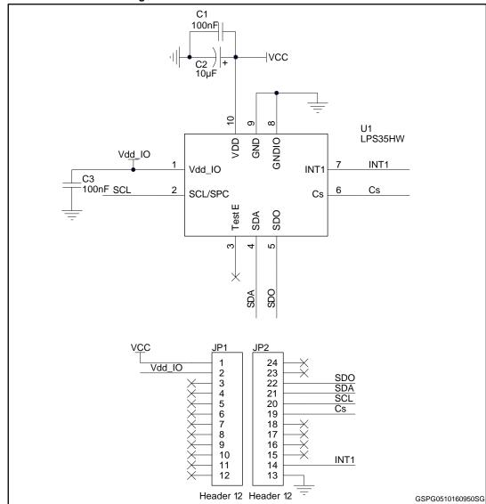
Figure 1: STEVAL-MKI177V1 circuit schematic
