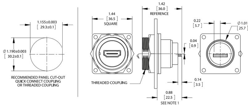
NOTE 1: THE DIMENSION DOES NOT INCLUDE GASKET COMPRESSION. NOTE 2: THE PINOUT IS TYPICAL FOR THREADED OR QUICK CONNECT COUPLING.
