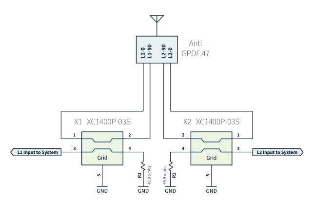
**Figure 1.** Schematic representation of GPDF.47.8.A.02 feed network. The pin numbers of hybrid couplers X1 and X2 follow the manufacturer's datasheet reference.
