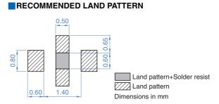
\* Make sure to connect the GND terminal of this product and the GND of the mounting circuit board by using through holes so that the distance between them is the shortest.
