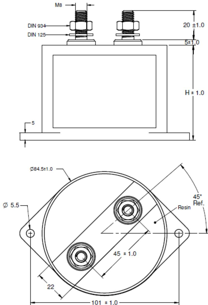
Lateral brackets for fixing are standard for all types.
