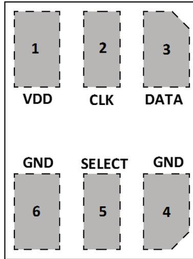
Figure 3. Pin Configuration Bottom View, Terminal Side Up)
