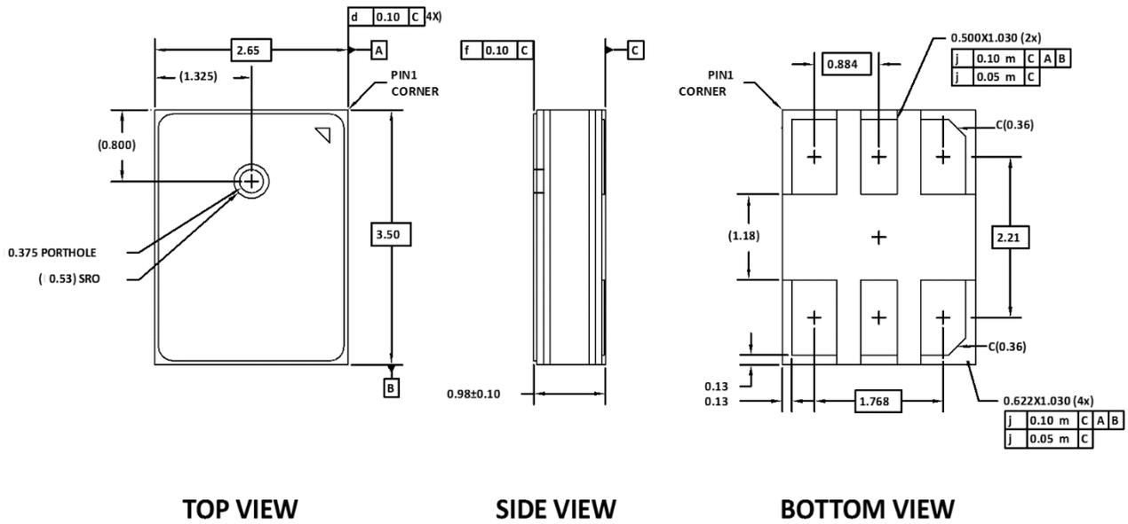
**Figure 116. 6-Terminal Chip Array Small Outline No-Lead Cavity**
