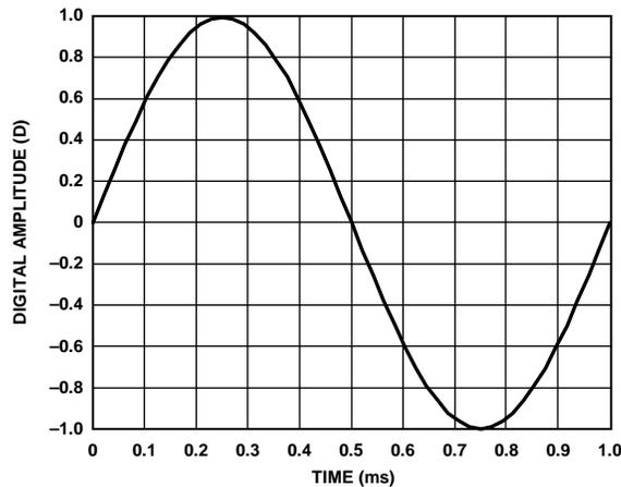
**Figure 10. 1 kHz, 0 dB FS Sine Wave**
