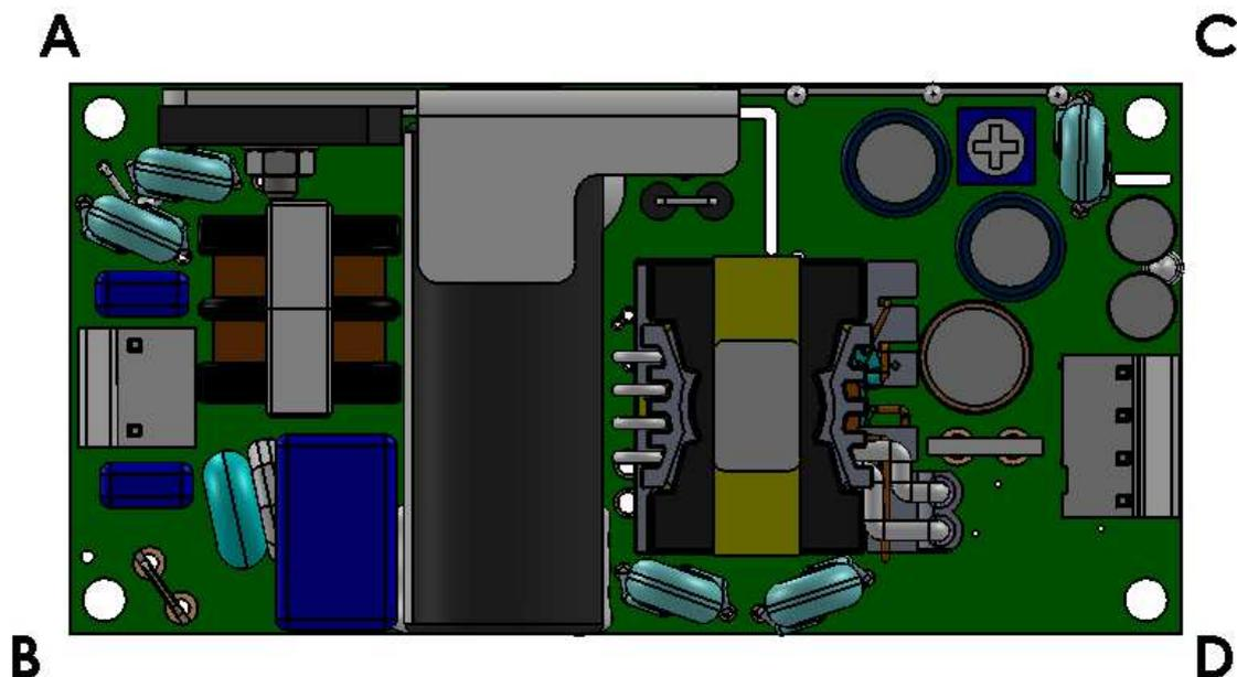
All four mounting points should be used to support the unit.
