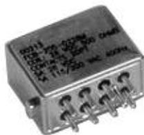
The Series FCB-205 relay is a polarized single-side stable design, where the flux from a permanent magnet provides the armature holding force in the deactivated state, and its flux path is switched and combined with the coil flux in the operated state. This results in appreciably
