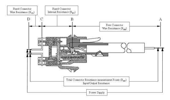
Jack-plug interface resistance:  $R_I = R_B = R_{AD} - (R_{AB} + R_{BD})$  [for reference only] IDC-wire interface resistance:  $R_I = R_C = R_{AD} - (R_{AC} + R_{CD})$  [for reference only] Connector Assembly Contact Resistance;  $\Delta R = R_{AD \, (initial)} - R_{AD \, (final)}$
