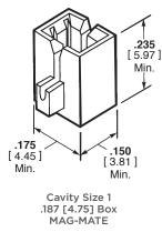
(Application Spec. 114-2069) Dimensions shown as in [mm].
