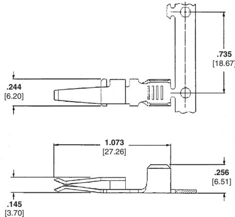
**Wire barrel accepts one 14, 16 or 18 AWG stranded copper conductor**
