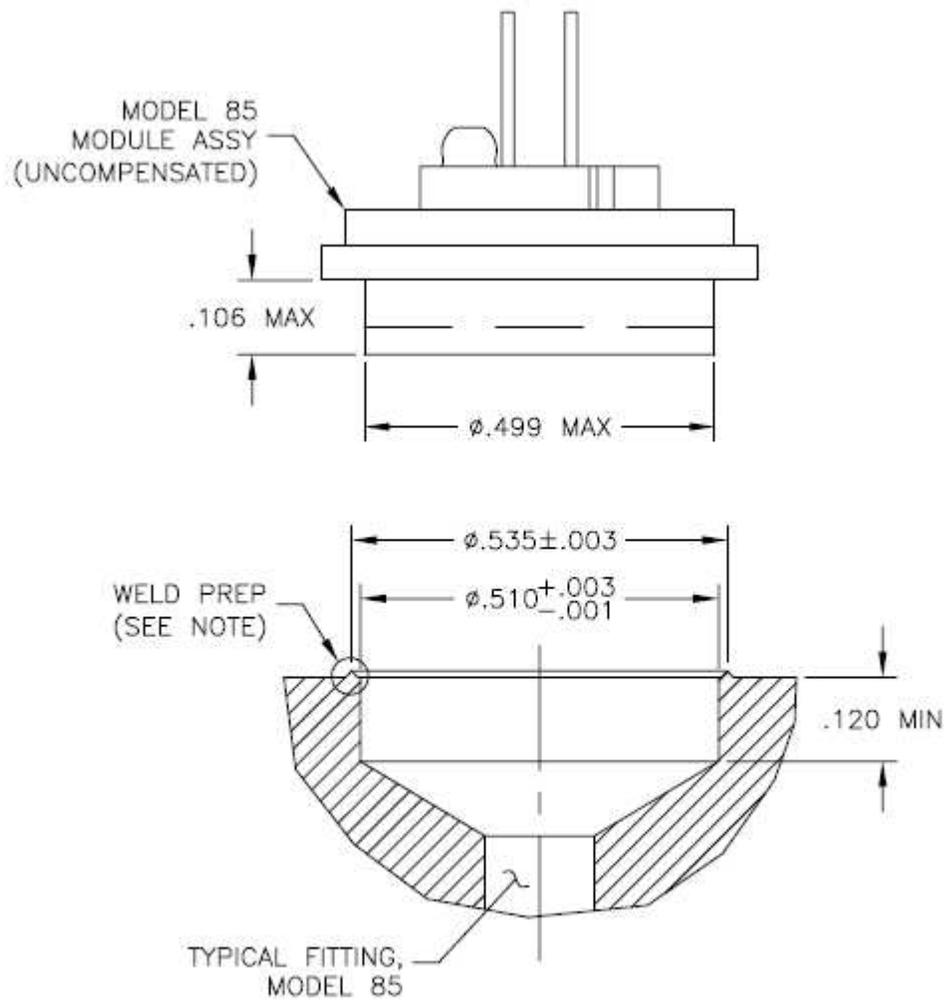
NOTE: WELD PREP SHOWN IS FOR RESISTANCE WELD. ACTUAL GEOMETRY VARIES PER CUSTOMER REQUIREMENTS.
