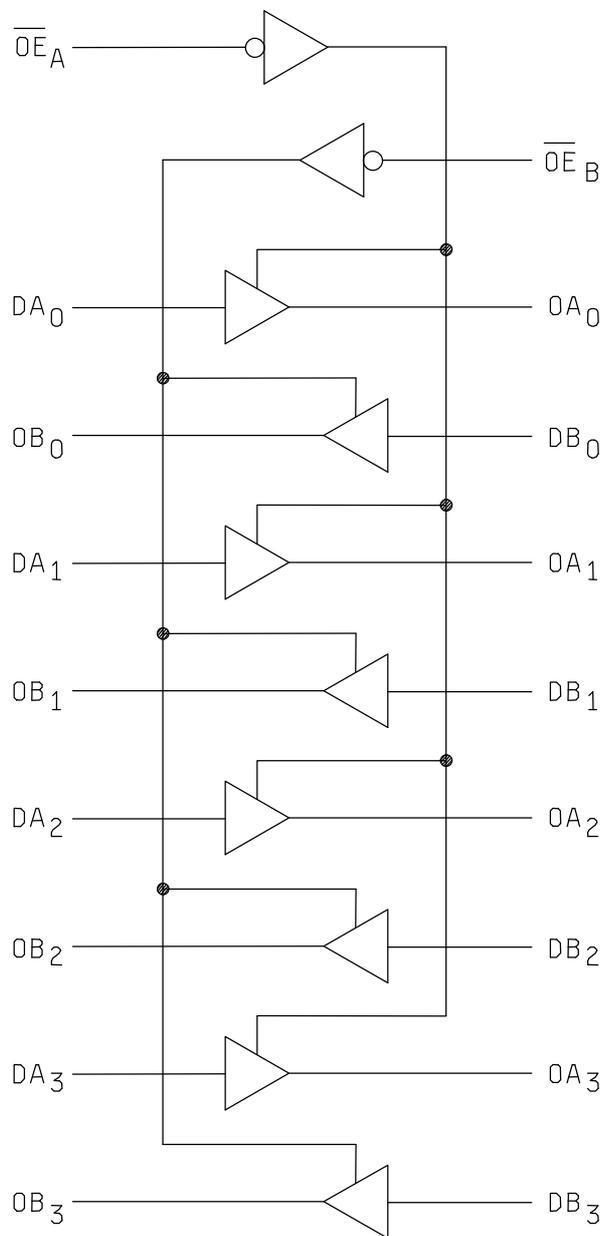
FIGURE 3. Logic diagram.
