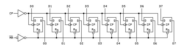
FIGURE 3. Logic diagram.
