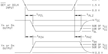
FIGURE 4. Switching waveforms and test circuit.
