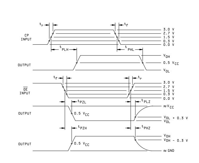
FIGURE 4. Switching waveforms and test circuit.
