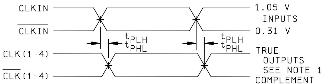
PROPAGATION DELAY, CLKIN/CLKIN TO OUTPUTS
