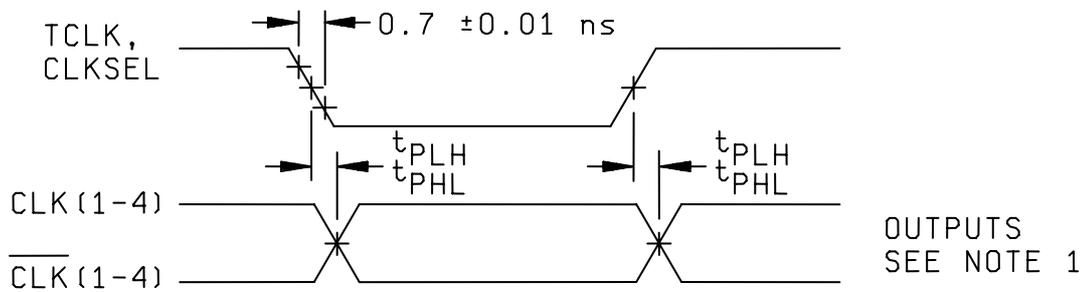
PROPAGATION DELAY, TCLK/CLKSEL TO OUTPUTS
