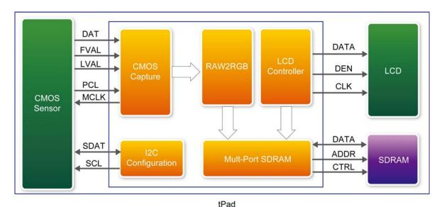
Figure 4-12 Block diagram of the digital camera design
