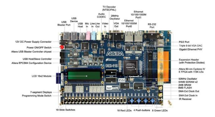
Figure 2-2 VEEK PCB and component diagram (bottom view)
