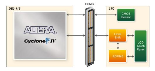
Figure 2-3 Block Diagram of VEEK
