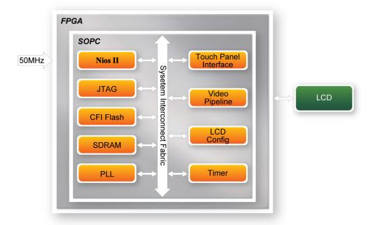
Figure 4-2 Block diagram of the VEEK Starter demonstration
