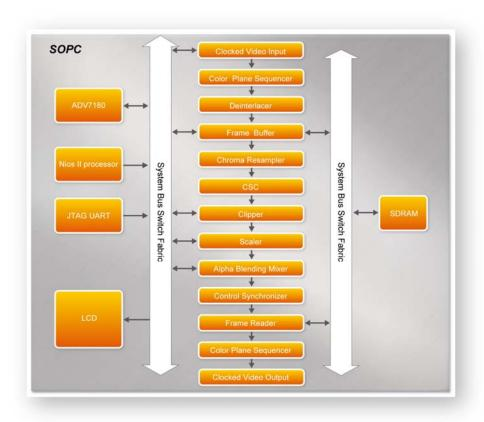
Figure 4-9 VIP Example SOPC Block Diagram (Key Components)
