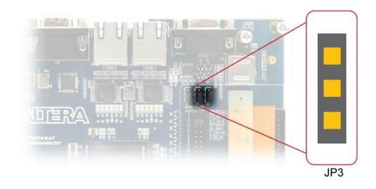
Figure 3-2 The JTAG chain configuration header
