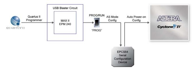
Figure 3-5 The AS configuration scheme
