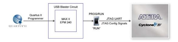
Figure 3-3 The JTAG chain configuration scheme
