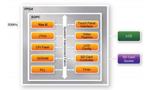
Figure 4-7 Block diagram of the picture viewer demonstration
