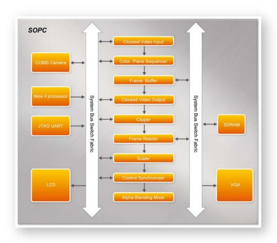
Figure 4-14 VIP Camera Example SOPC Block Diagram (Key Components)
