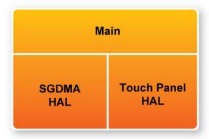
Figure 4-3 Software stack of the VEEK Starter demonstration
