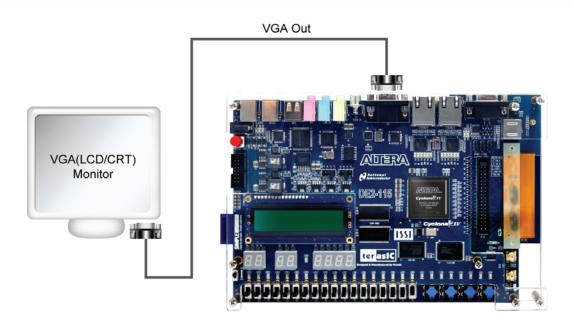
Figure 4-15 Setup for the VEEK\_VIP\_Camera demonstration
