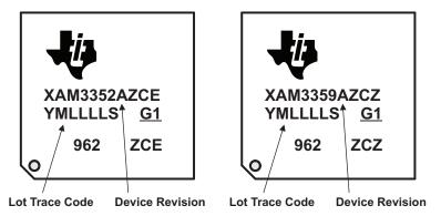
Figure 1. Example of Device Revision Codes for the AM335x Microprocessor
