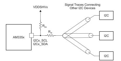
Figure 4. Placement of Series Termination Resistor and Pullup Resistor
