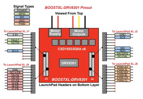
Figure 2: BOOSTXL-DRV8301 Pinout
