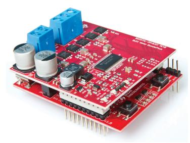
Figure 1: BOOSTXL-DRV8301 On Top LaunchPad
